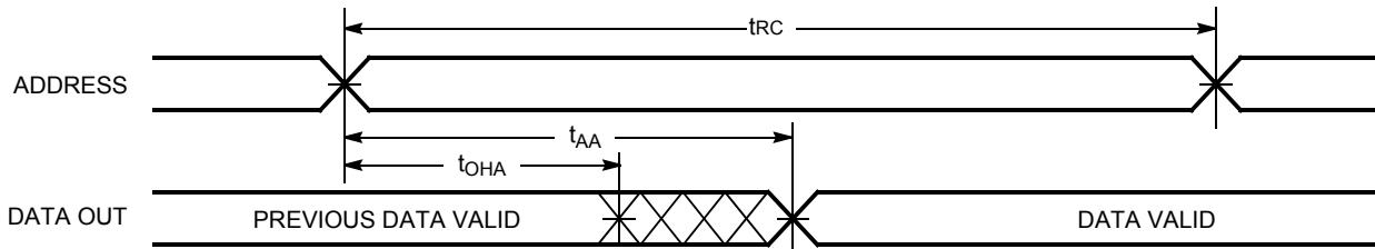
**Figure 5. Read Cycle No. 2 ( $\overline{OE}$  Controlled) [16, 17]**
