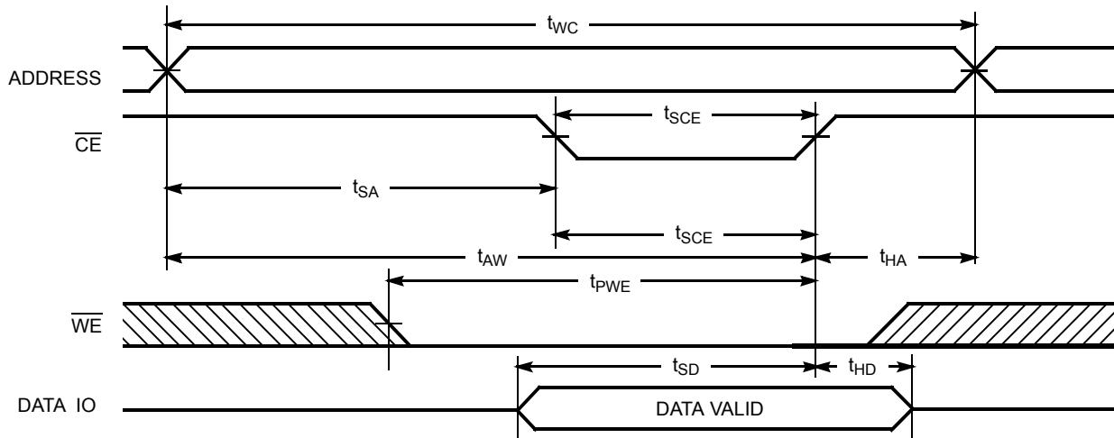
**Figure 7. Write Cycle No. 2 ( $\overline{\text{WE}}$  Controlled,  $\overline{\text{OE}}$  HIGH During Write) [18, 19]**
