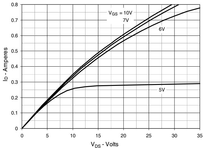
**Fig. 2. Output Characteristics @  $T_J = 125^\circ\text{C}$**
