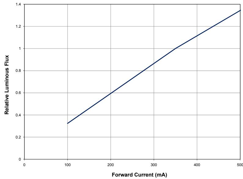
Figure 7. Typical relative luminous flux vs. forward current.
