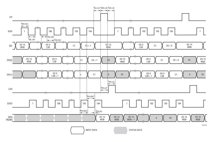
Figure 3. Serial Data Input and Output Timing Chart
