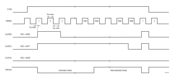
Figure 4. Grayscale PWM Dimming and Precharging Signal Timing Chart
