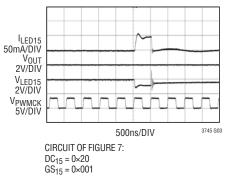
200Hz Two-Level DC Dimming
