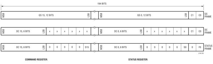
C1: ENABLE LED CHANNELS - ENABLE = 1, DISABLE = 0 C0: FRAME SELECT - GS FRAME = 0, DC FRAME = 1 S0-S15: LED 0-15 FAULT - FAULT = 1, 0K = 0 F0: 0T - 0VER TEMPERATURE = 1, 0K = 0
