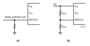
Figure 6. Methods of Controlling the EN/UVLO Pin
