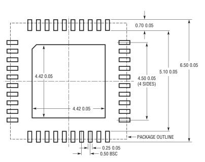
UJ Package 40-Lead Plastic QFN (6mm × 6mm) (Reference LTC DWG # 05-08-1728 Rev Ø)
