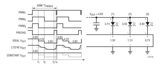
Figure 5. Adaptive-Tracking-Plus-Precharging LED Bus Voltage Technique
