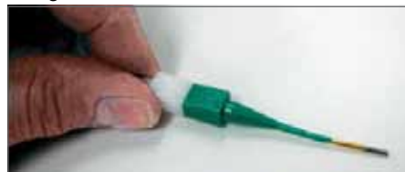
Plastic tool with contact in proper position.
