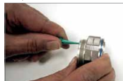
Plastic tool with contact in proper position.
