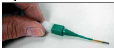
Plastic tool with contact in proper position.
