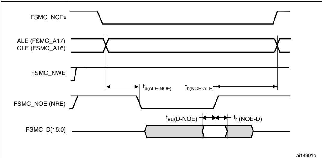
**Figure 69. NAND controller waveforms for write access**
