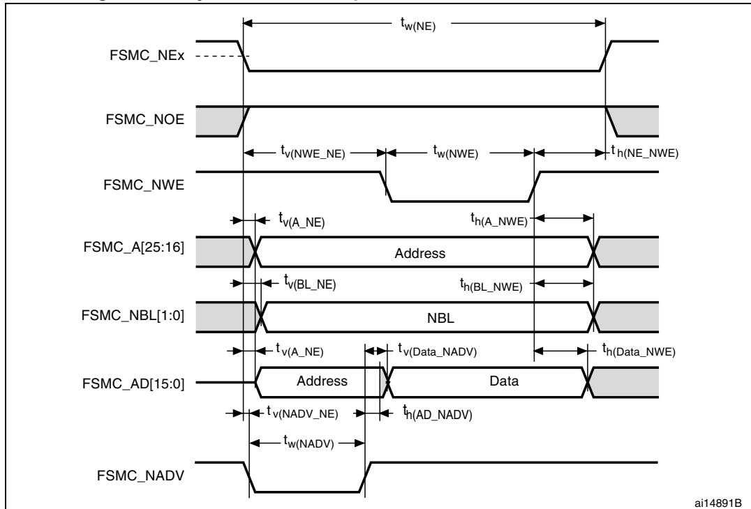
**Table 78. Asynchronous multiplexed PSRAM/NOR write timings<sup>(1)(2)</sup>**
