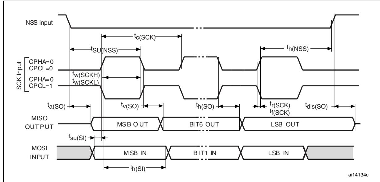
Figure 40. SPI timing diagram - slave mode and CPHA = 1
