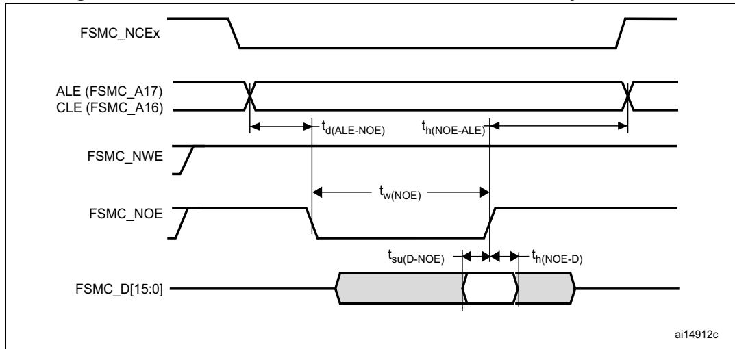
**Figure 71. NAND controller waveforms for common memory write access**
