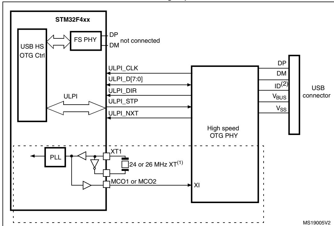
1. It is possible to use MCO1 or MCO2 to save a crystal. It is however not mandatory to clock the STM32F41xxx with a 24 or 26 MHz crystal when using USB HS. The above figure only shows an example of a possible connection.
