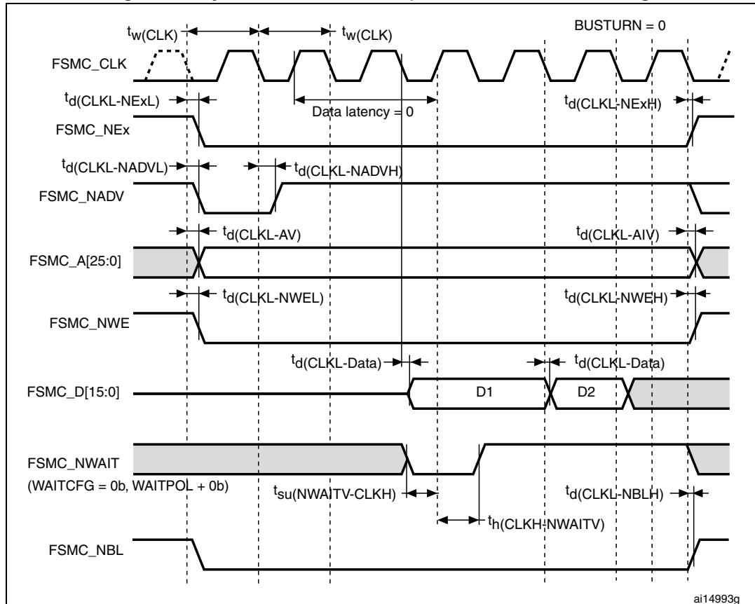
Table 82. Synchronous non-multiplexed PSRAM write timings<sup>(1)(2)</sup>
