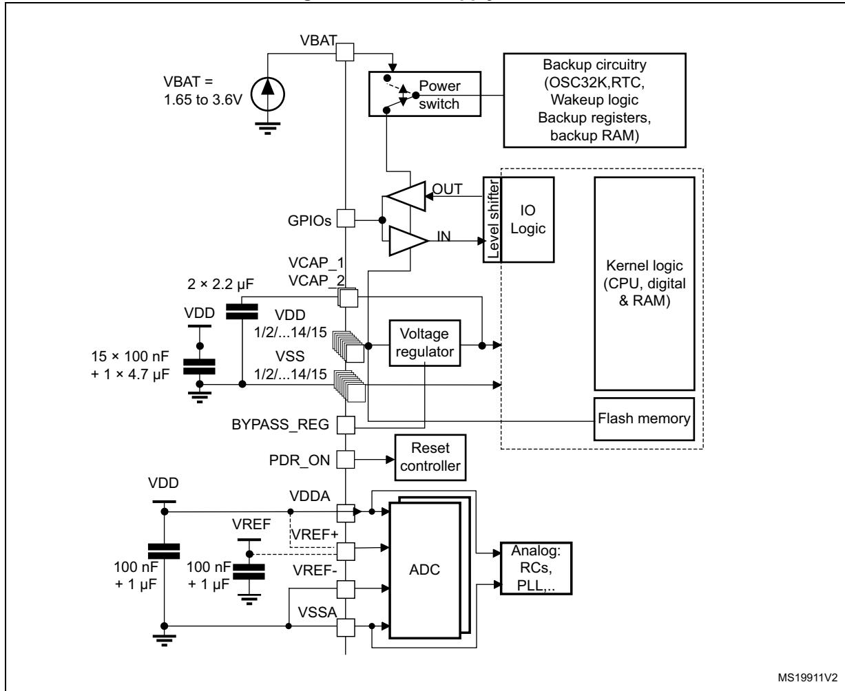
1. Each power supply pair must be decoupled with filtering ceramic capacitors as shown above. These capacitors must be placed as close as possible to, or below, the appropriate pins on the underside of the PCB to ensure the good functionality of the device.
