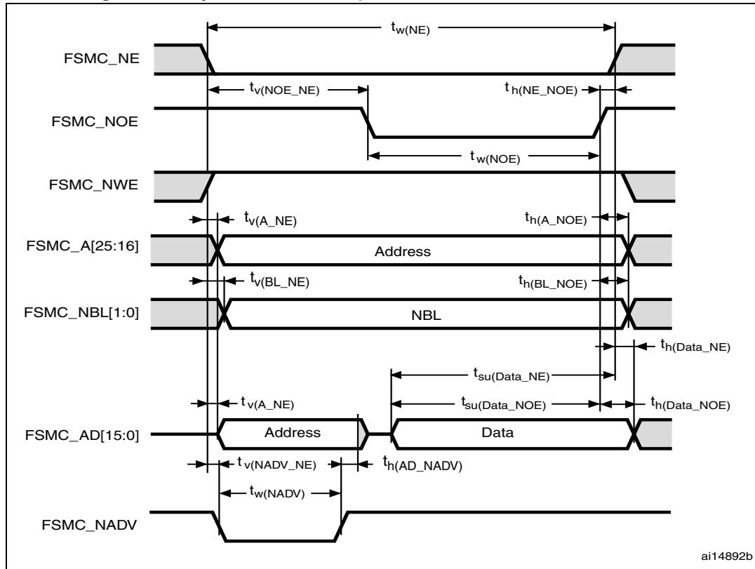
Table 77. Asynchronous multiplexed PSRAM/NOR read timings<sup>(1)(2)</sup>
