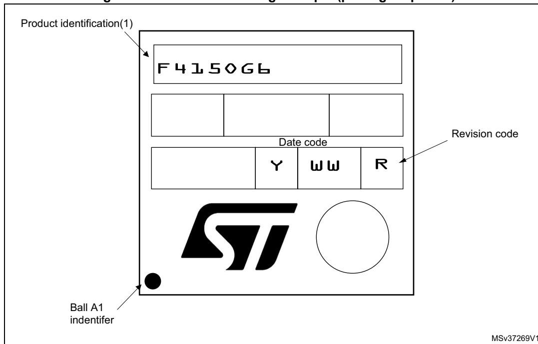
1. Parts marked as "ES", "E" or accompanied by an Engineering Sample notification letter, are not yet qualified and therefore not yet ready to be used in production and any consequences deriving from such usage will not be at ST charge. In no event, ST will be liable for any customer usage of these engineering samples in production. ST Quality has to be contacted prior to any decision to use these Engineering Samples to run qualification activity.
