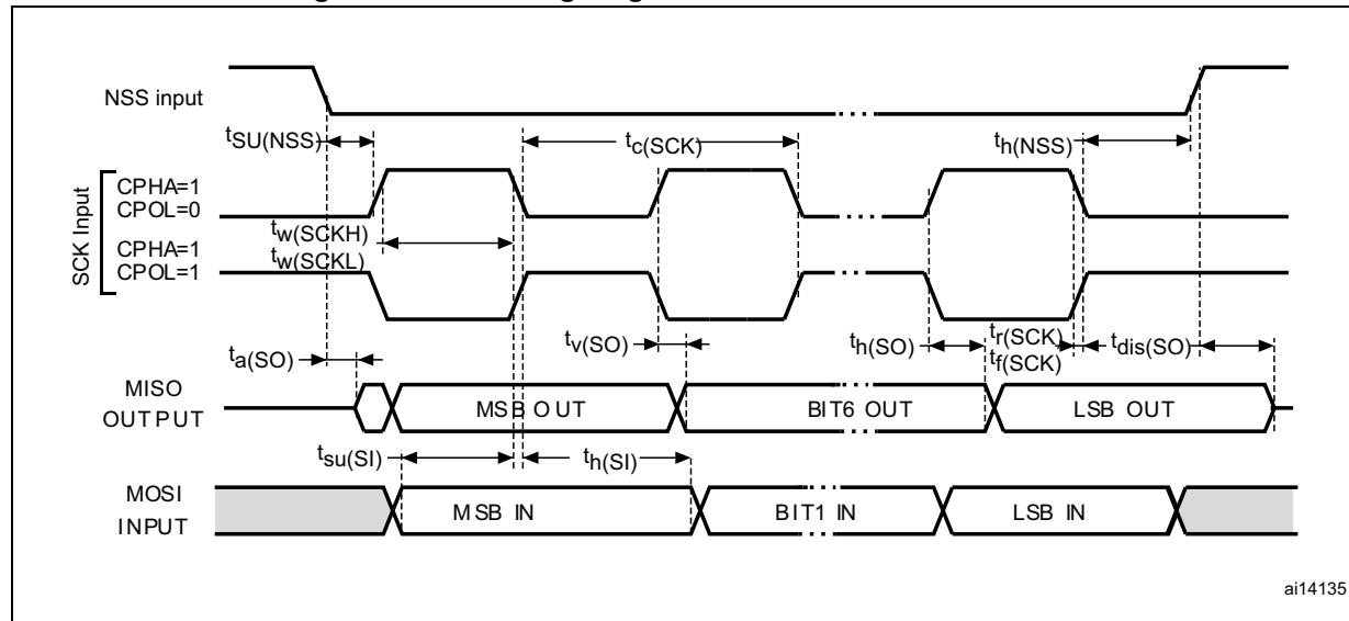
Figure 41. SPI timing diagram - master mode
