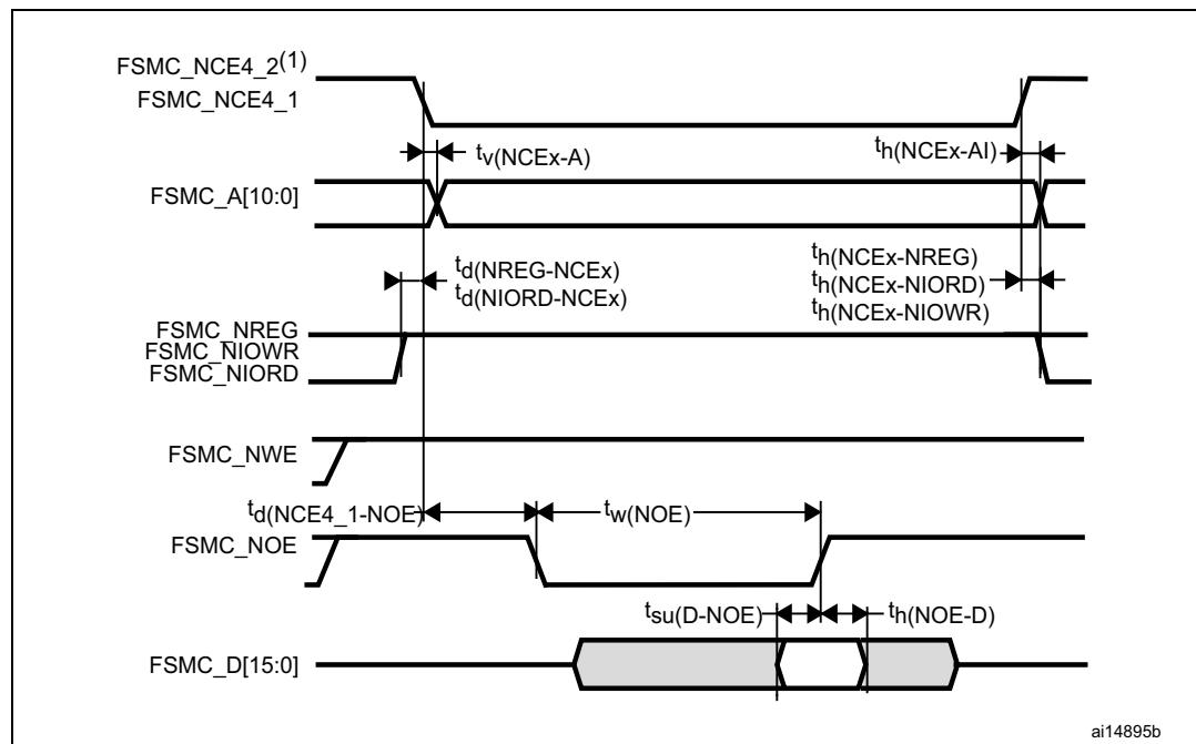
1. FSMC\_NCE4\_2 remains high (inactive during 8-bit access).
