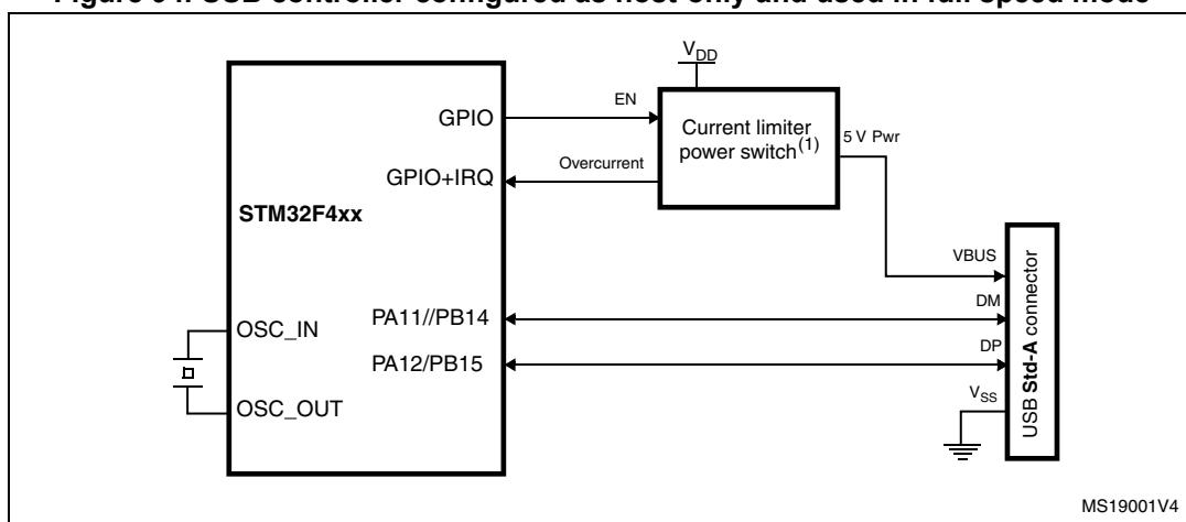
1. The current limiter is required only if the application has to support a V<sub>BUS</sub> powered device. A basic power switch can be used if 5 V are available on the application board.
