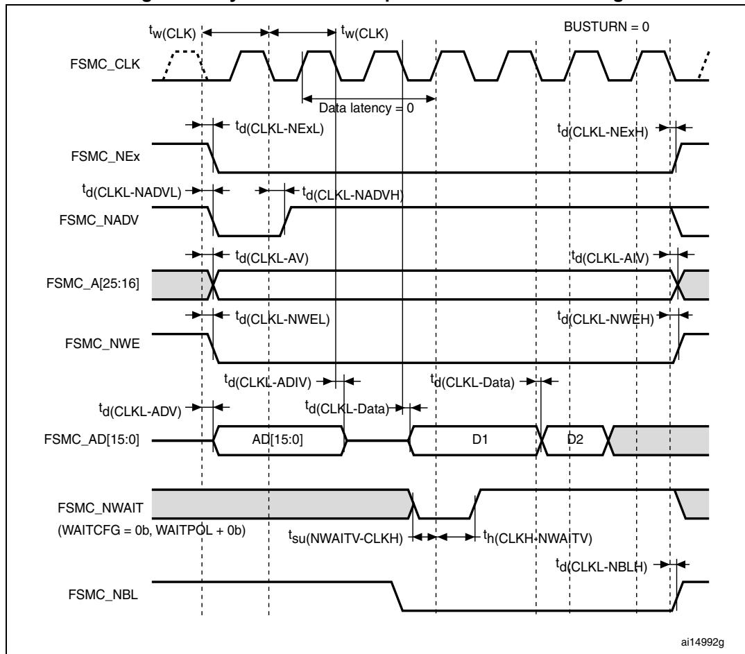
Table 80. Synchronous multiplexed PSRAM write timings<sup>(1)(2)</sup>
