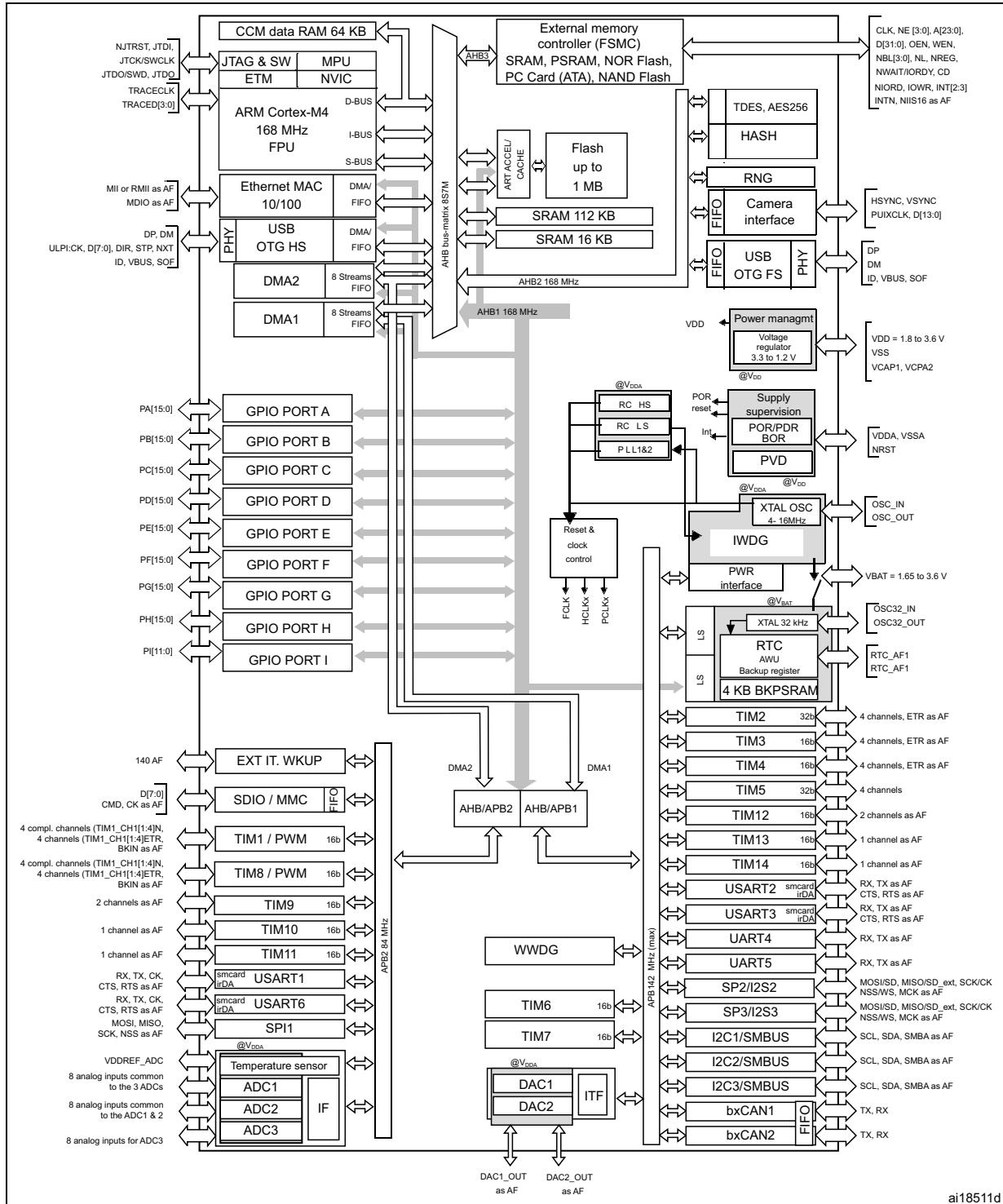
1. The timers connected to APB2 are clocked from TIMxCLK up to 168 MHz, while the timers connected to APB1 are clocked from TIMxCLK either up to 84 MHz or 168 MHz, depending on TIMPRE bit configuration in the RCC\_DCKCFGR register.
