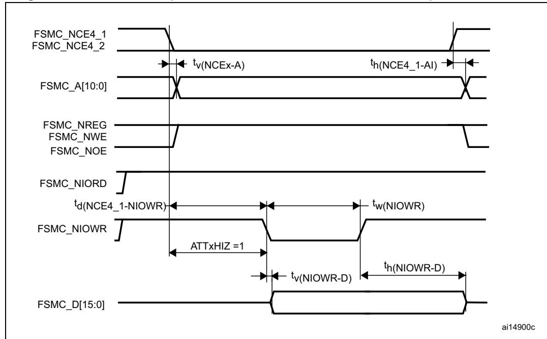
Table 83. Switching characteristics for PC Card/CF read and write cycles in attribute/common space<sup>(1)(2)</sup>
