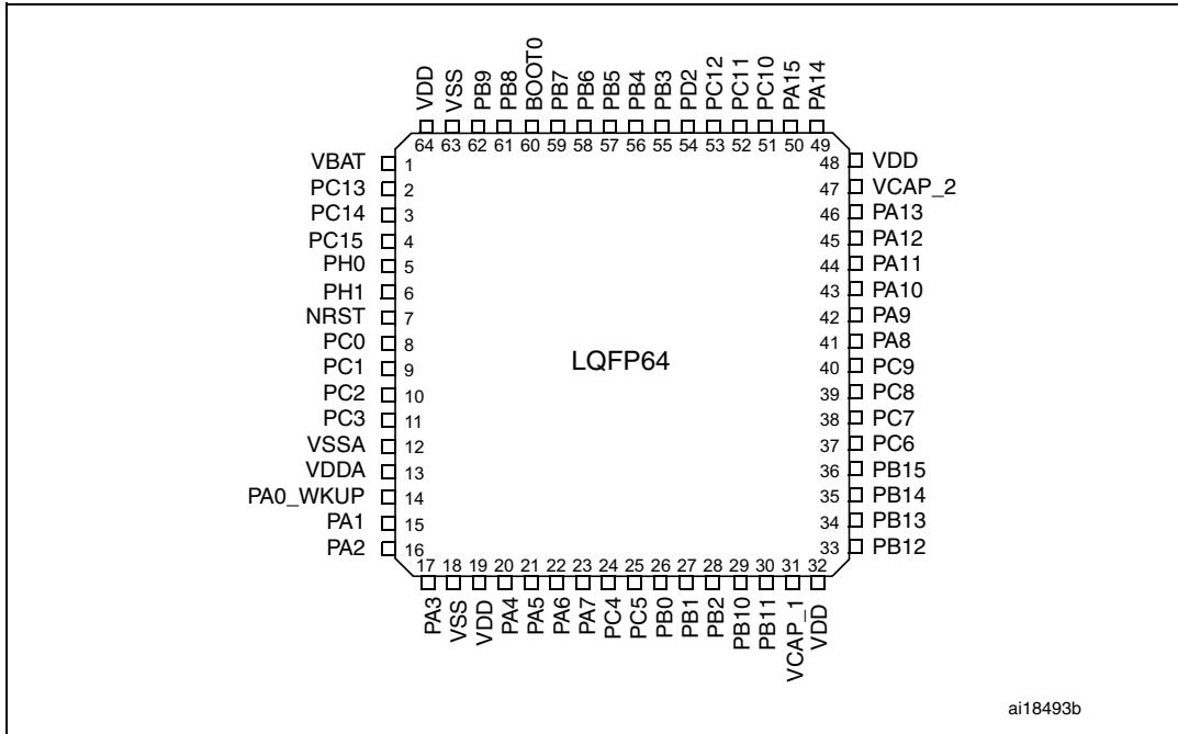
1. The above figure shows the package top view.
