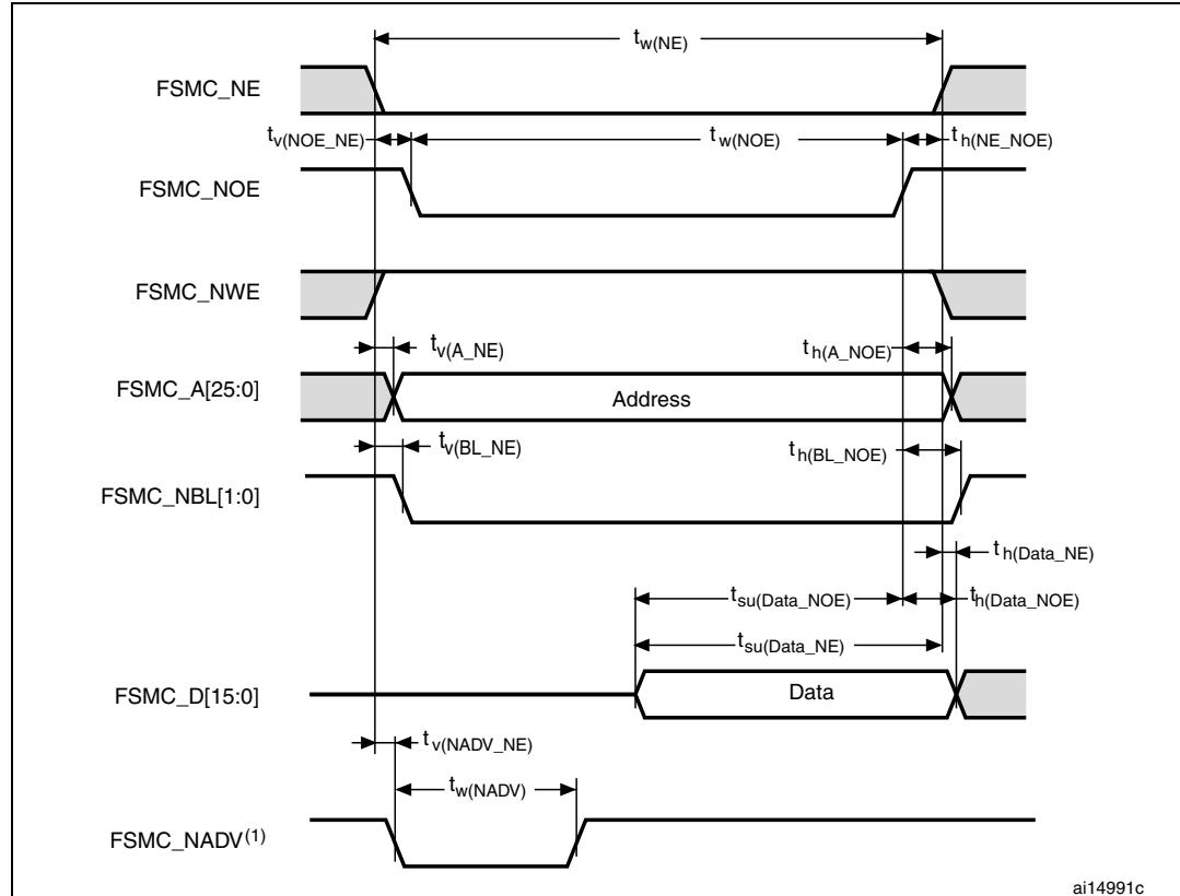
1. Mode 2/B, C and D only. In Mode 1,  $\text{FSMC\_NADV}$  is not used.
