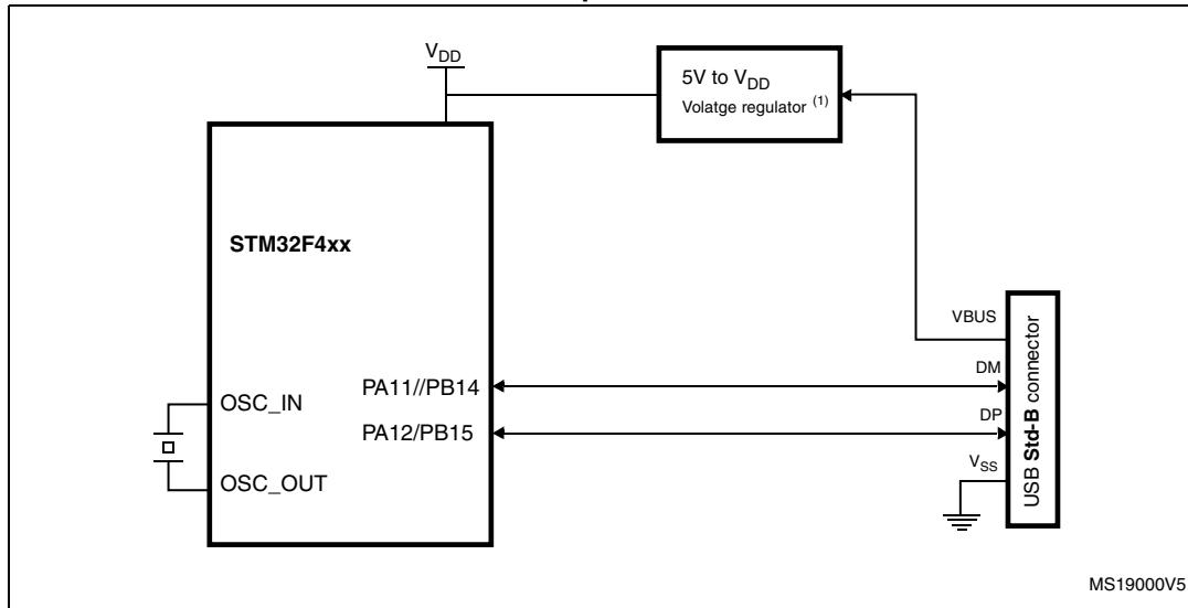
1. External voltage regulator only needed when building a V<sub>BUS</sub> powered device.
