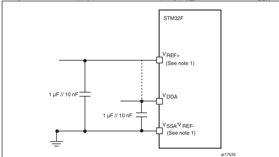
1.  $V_{REF+}$  and  $V_{REF-}$  inputs are both available on UFBGA176.  $V_{REF+}$  is also available on LQFP100, LQFP144, and LQFP176. When  $V_{REF+}$  and  $V_{REF-}$  are not available, they are internally connected to  $V_{DDA}$  and  $V_{SSA}$ .
