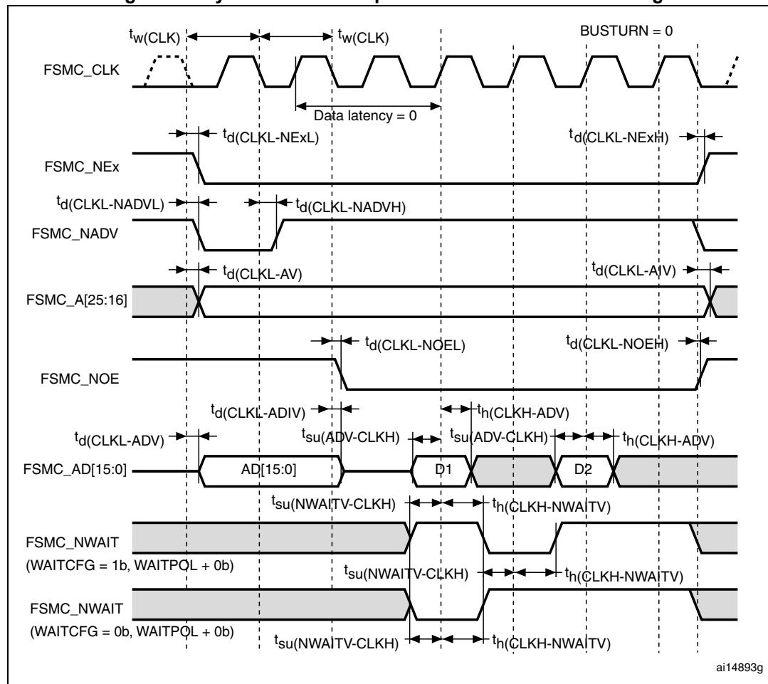
**Table 79. Synchronous multiplexed NOR/PSRAM read timings<sup>(1)(2)</sup>**
