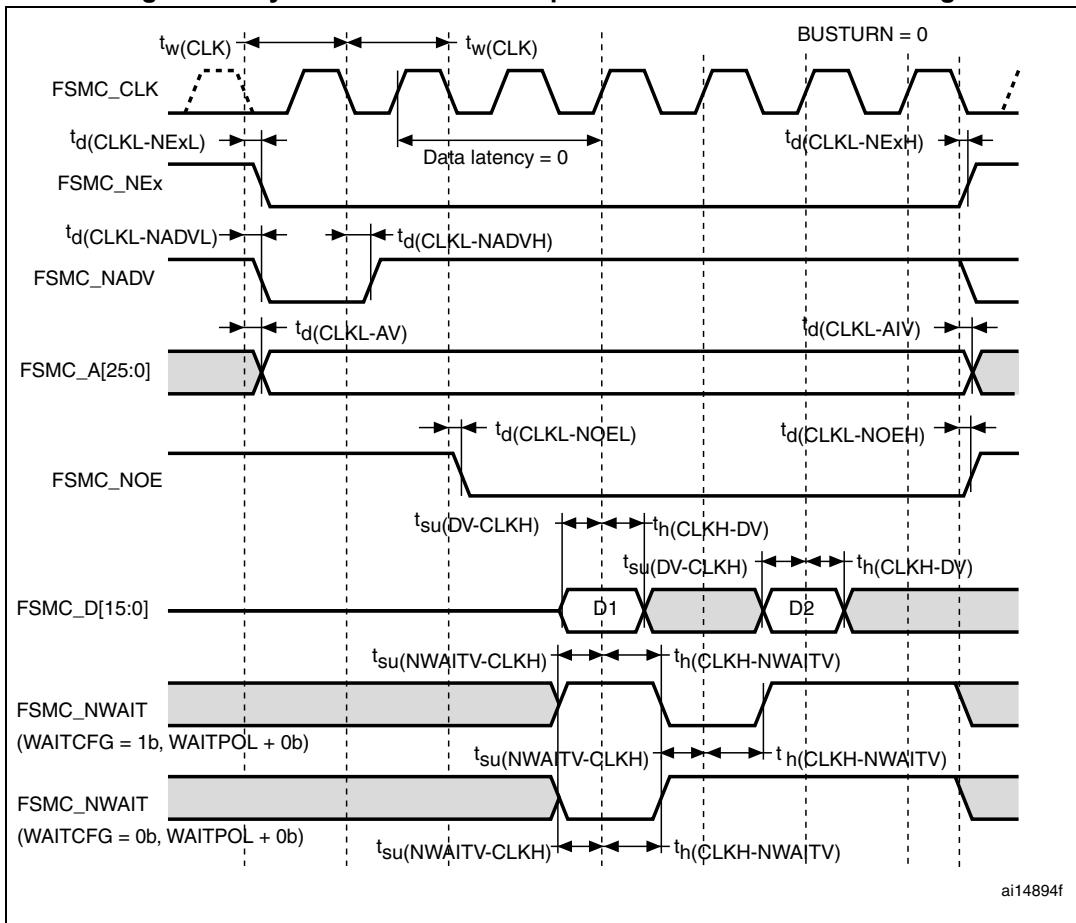
**Table 81. Synchronous non-multiplexed NOR/PSRAM read timings<sup>(1)(2)</sup>**
