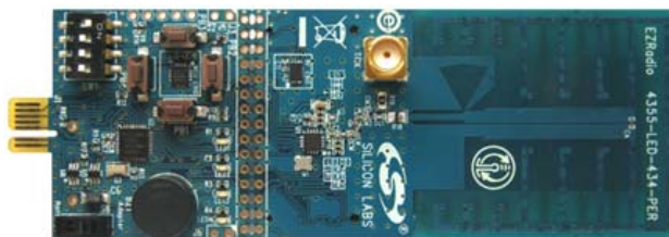
Figure 2. Si4355 RFStick 434 MHz Receiver Board (P/N 4355-LED-434-SRX)
