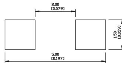
Recommended Soldering Pattern For Reflow Soldering
