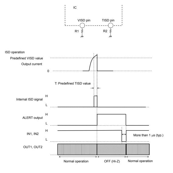
Note: The ISD circuit is activated if the absolute maximum current rating is violated. Note that the circuit is provided as an auxiliary only and does not necessarily provide the IC with a perfect protection from damages due to overcurrent caused by power fault, ground fault, load-short and the like.
