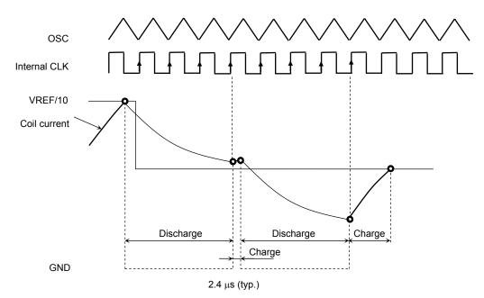
(4) Operation on change of predetermined current value (when in Charge mode) Even though VREF reaches the predetermined current value, Discharge mode continues for four internal clocks after that. And then Charge mode is entered.
