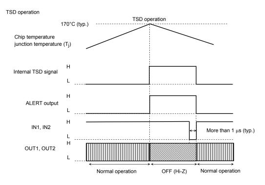
Note: The TSD circuit is activated if the absolute maximum junction temperature rating (T<sub>j</sub>) of 150°C is violated. Note that the circuit is provided as an auxiliary only and does not necessarily provide the IC with a perfect protection from any kind of damages.
