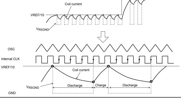
(3) Operation on change of predetermined current value (when in Discharge mode) The TB6569FG enters Discharge mode as V<sub>RSGND</sub> reaches the predetermined voltage (VREF/10) and then transits to Charge mode after four internal clocks. However, if V<sub>RSGND</sub> > VREF/10 at the time, the TB6569FG goes back to Discharge mode. If V<sub>RSGND</sub> > VREF/10 after another four internal clocks, then the TB6569FG enters Charge mode and stays until V<sub>RSGND</sub> reaches VREF/10.
