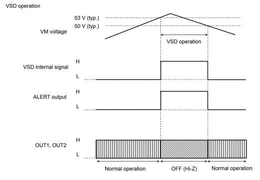
Note: The VSD circuit is activated if the absolute maximum voltage rating is violated. Note that the circuit is provided as an auxiliary only and does not necessarily provide the IC with a perfect protection from any kind of damages.
