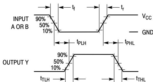
Figure 1. Switching Waveforms
