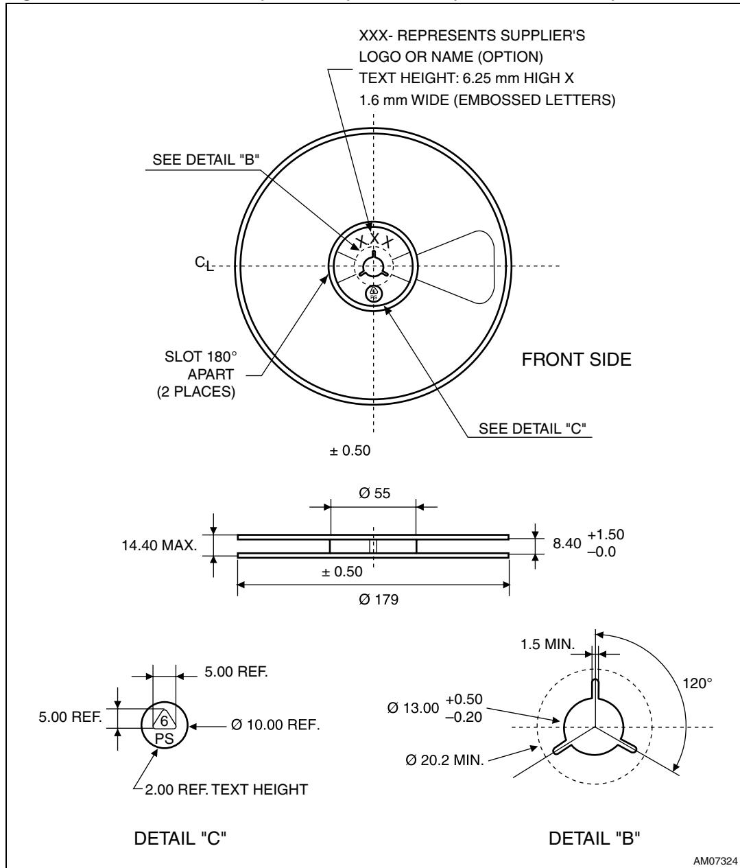
**Figure 9. Reel information (back view) for QFN10 (1.8 x 1.4 x 0.5 mm)**
