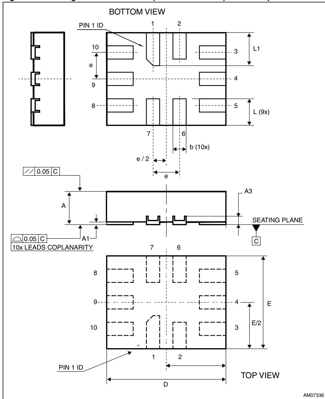
**Table 7. Mechanical data for QFN10 (1.8 x 1.4 x 0.5 mm) - 0.40 mm pitch**
