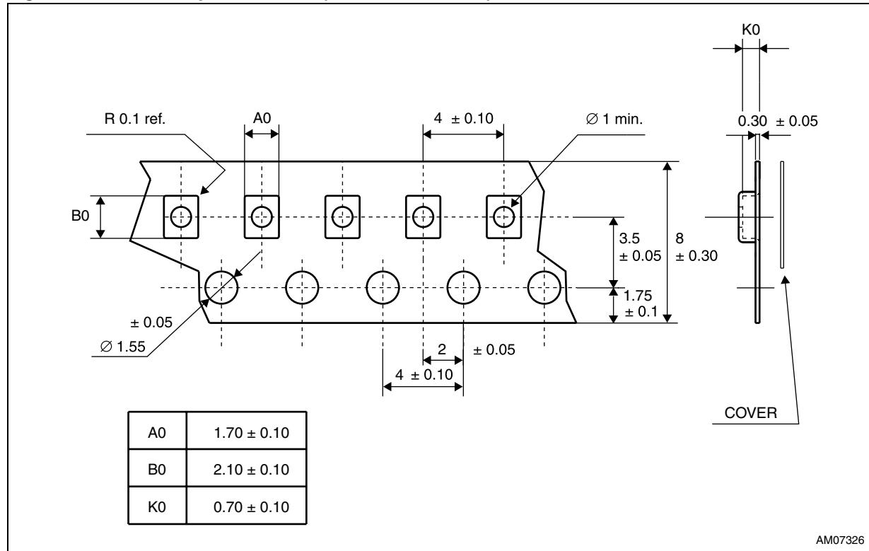
Figure 8. Reel information (front side) for QFN10 (1.8 x 1.4 x 0.5 mm)
