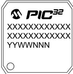
100-Lead TQFP (12x12x1 mm)
