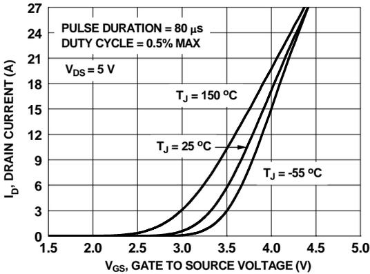
**Figure 5. Transfer Characteristics**
