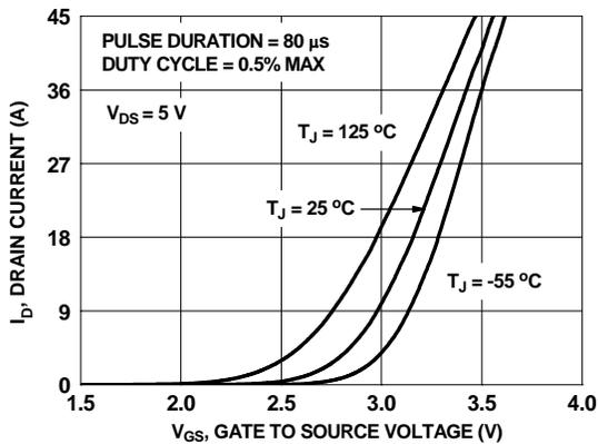
Figure 17. Transfer Characteristics
