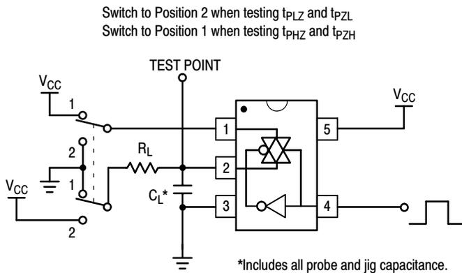
Figure 8. Propagation Delay Output Enable/Disable Test Set-Up
