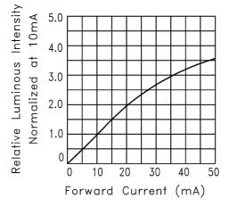
Fig.4 RELATIVE LUMINOUS INTENSITY VS. FORWARD CURRENT
