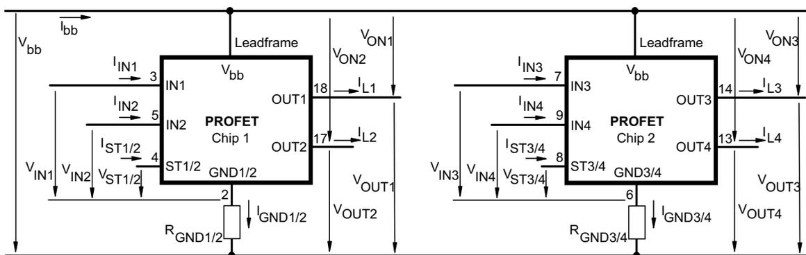
Leadframe ( $V_{bb}$ ) is connected to pin 1,10,11,12,15,16,19,20
