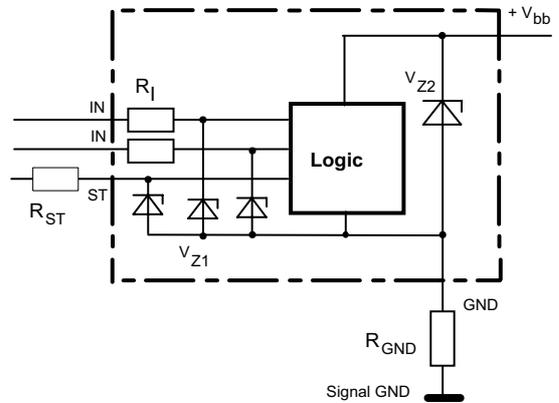
$V_{Z1} = 6.1 \text{ V typ.}, V_{Z2} = 47 \text{ V typ.}, R_1 = 3.5 \text{ k}\Omega \text{ typ.}, R_{GND} = 150 \Omega$
