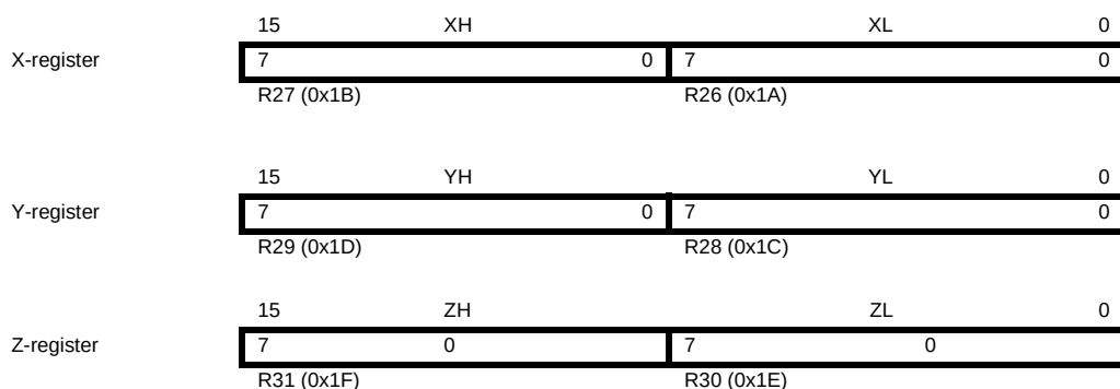
Figure 5-3. The X-, Y-, and Z-registers
