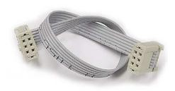
Note: Pin no. 1 is signed by triangle scratch on ISP cable connectors.
