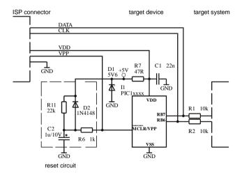
**Note:** External reset circuit is necessary only if VDD power-up slope is too slow.
