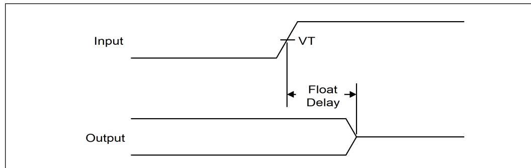
**Figure 10-16. Output Enable Delay**
