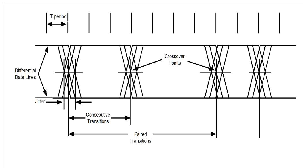
**Figure 10-10. USB EOP Width**
