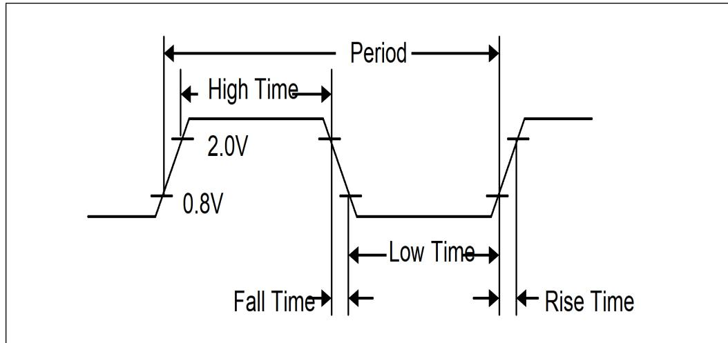
**Figure 10-5. Measurement Points for Differential Waveforms**
