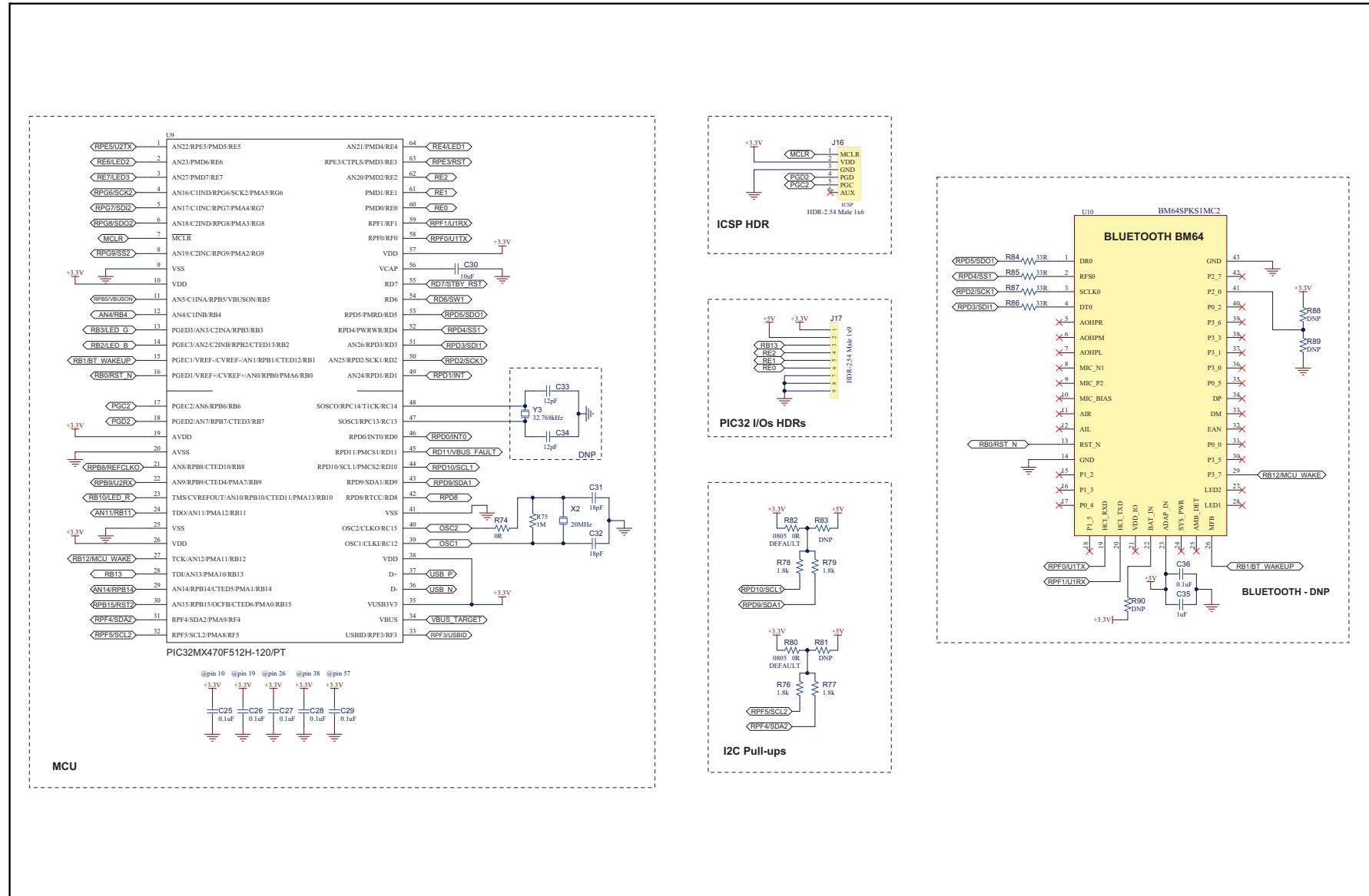
**FIGURE A-3: PIC32MX470 CURIOSITY DEVELOPMENT BOARDSHEET 2 OF 3**
