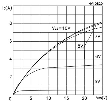
**Figure 4. Transfer characteristics**
