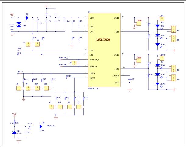
Figure 5: IS32LT3126 DEMO Schematic
