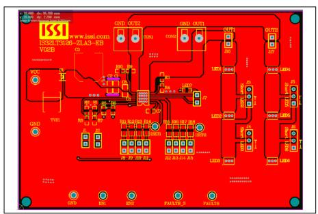
Figure 7 Board PCB Layout- Top Layer
