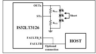
Figure 3 STx Pins Operation
