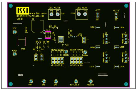
Figure 6 Board Component Placement Guide - Top Layer
