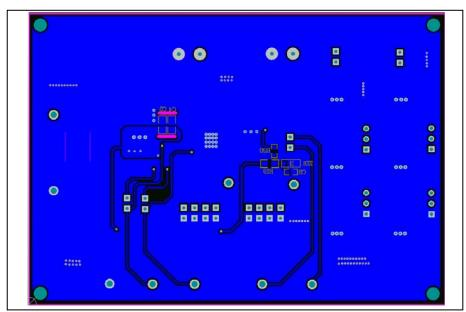
Figure 9 Board PCB Layout - Bottom Layer
