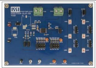
Figure 1: Photo of IS32LT3126 Evaluation Board
