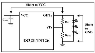
Figure 4 OUTx Pins Short Operation
