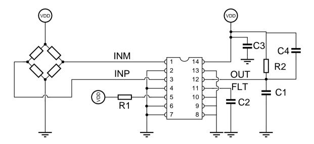
The external temperature sensor is only needed for applications where the temperature surrounding the customer sensor is different from the temperature surrounding the MLX90326. In the ratio-metric application mode, to keep the accuracy, the same supply should be used for the customer sensor, the MLX90326 and an ADC that makes the digital conversion of the analog output signal.
