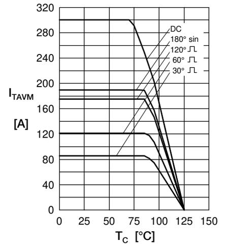
Fig. 3 Max. forward current at case temperature
