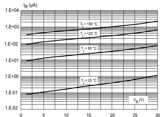
**Figure 6. Relative variation of reverse leakage current versus junction temperature (typical values)**
