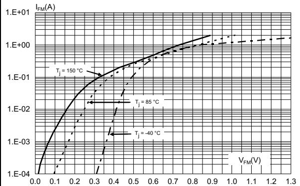
**Figure 9. Forward voltage drop versus forward current (typical values)**
