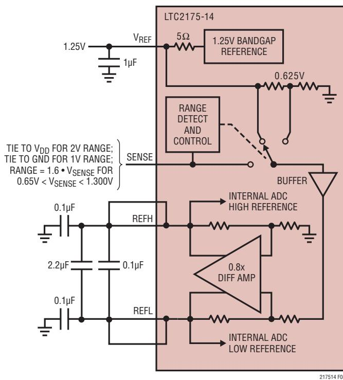
Figure 8. Reference Circuit
