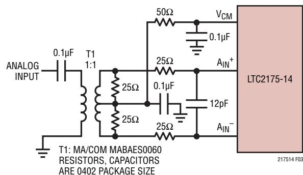
Figure 3. Analog Input Circuit Using a Transformer.
