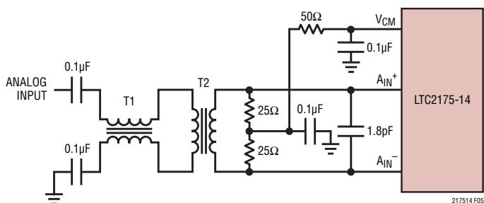
**Figure 5. Recommended Front End Circuit for Input Frequencies from 170MHz to 300MHz**
