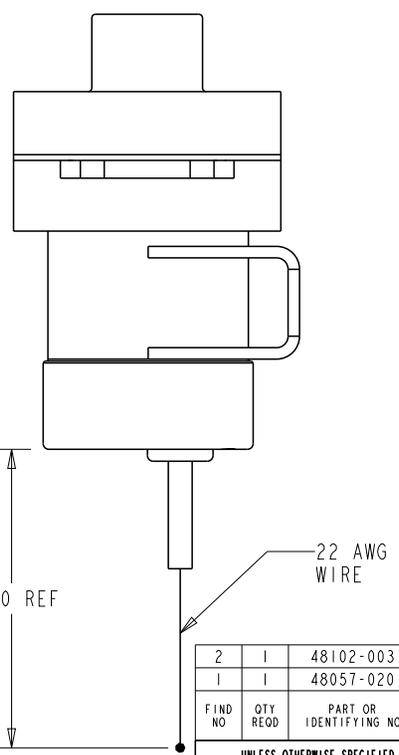
CONSTRUCTION MOUNTING STYLE: GASKET SEALED CHASSIS MOUNT
