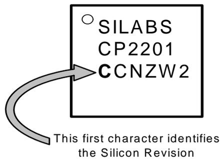
**Figure 31. Device Package—QFN 28**
