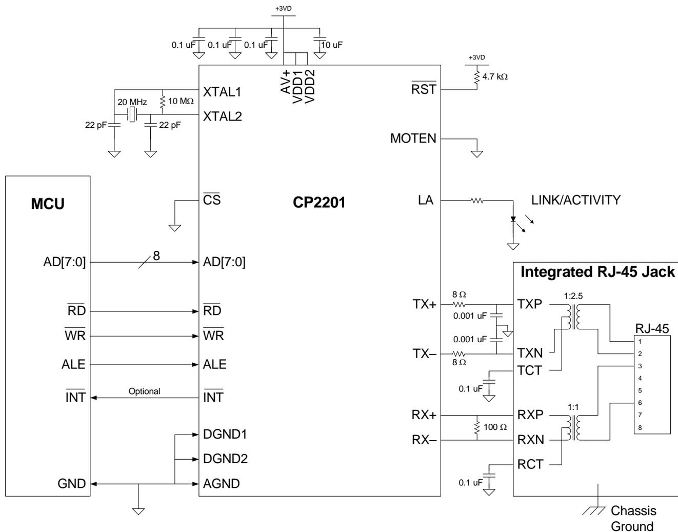
**Note:** The CP220x should be placed within 1 inch of the transformer for optimal performance.
