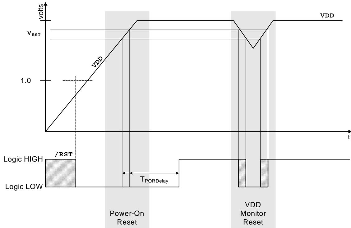
Figure 14. Reset Timing
