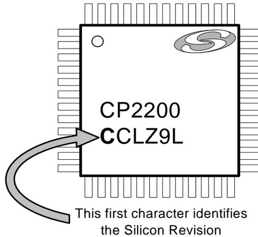
**Figure 30. Device Package—TQFP 48**
