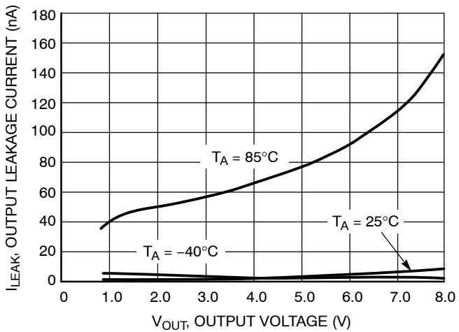
**Figure 14. NCS2202 Output Leakage Current versus Output Voltage**
