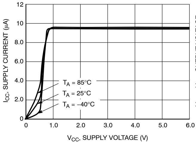
**Figure 3. NCS2200 Series Supply Current versus Supply Voltage**
