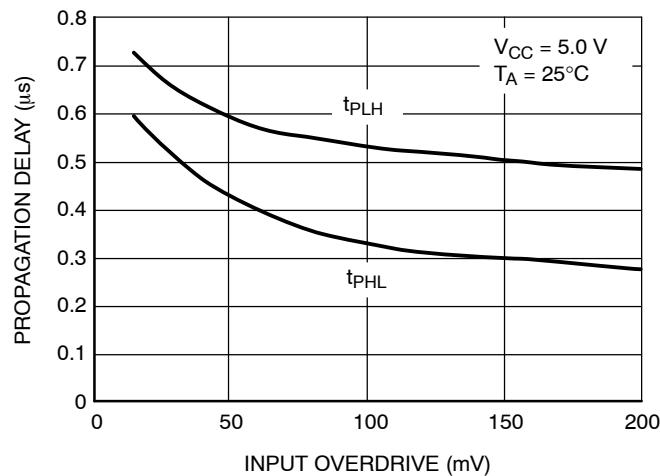
**Figure 11. NCS2200 Series Propagation Delay versus Input Overdrive**
