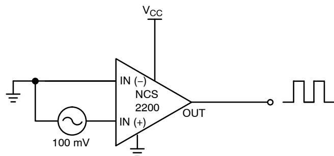
**Figure 21. Zero-Crossing Detector**
