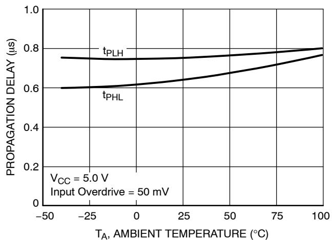
**Figure 8. NCS2200 Series Propagation Delay versus Temperature**
