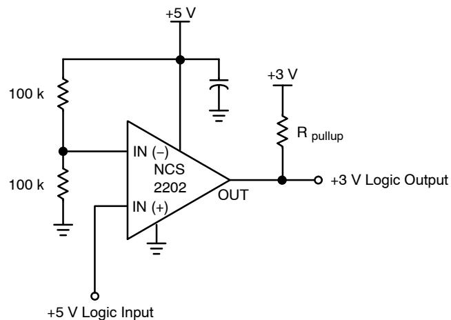
This circuit converts 5 V logic to 3 V logic. Using the NCS2202/3 allows for full 5 V logic swing without creating overvoltage on the 3 V logic input.
