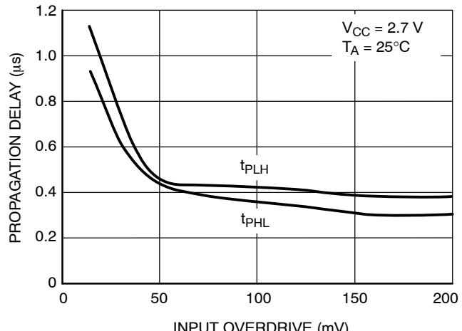
**Figure 10. NCS2200 Series Propagation Delay versus Input Overdrive**
