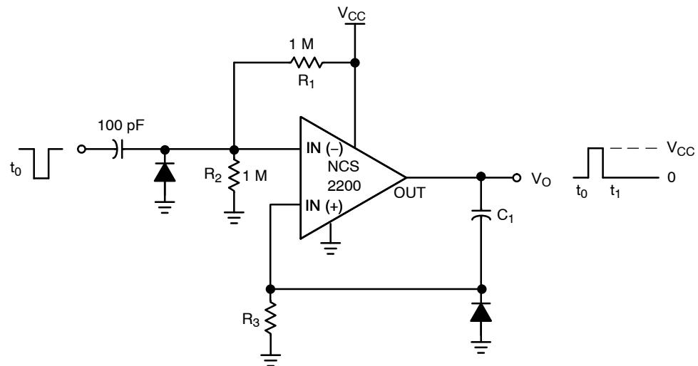
The resistor divider  $R_1$  and  $R_2$  can be used to set the magnitude of the input pulse. The pulse width is set by adjusting  $C_1$  and  $R_3$ .
