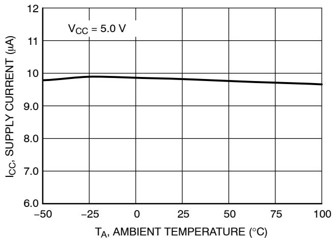
**Figure 1. NCS2200 Series Supply Current versus Temperature**
