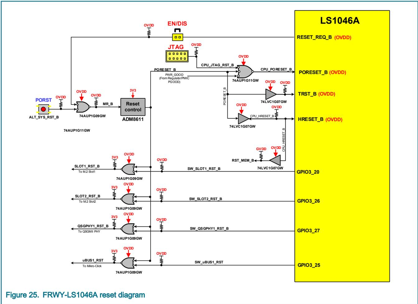
Figure 25. FRWY-LS1046A reset diagram
