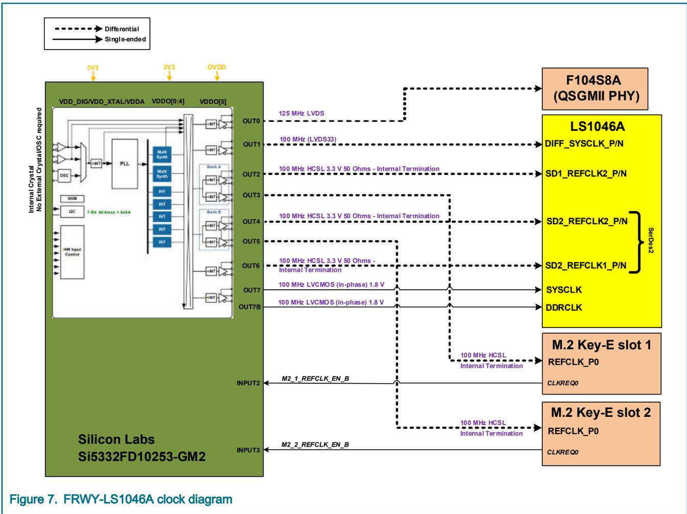
Figure 7. FRWY-LS1046A clock diagram
