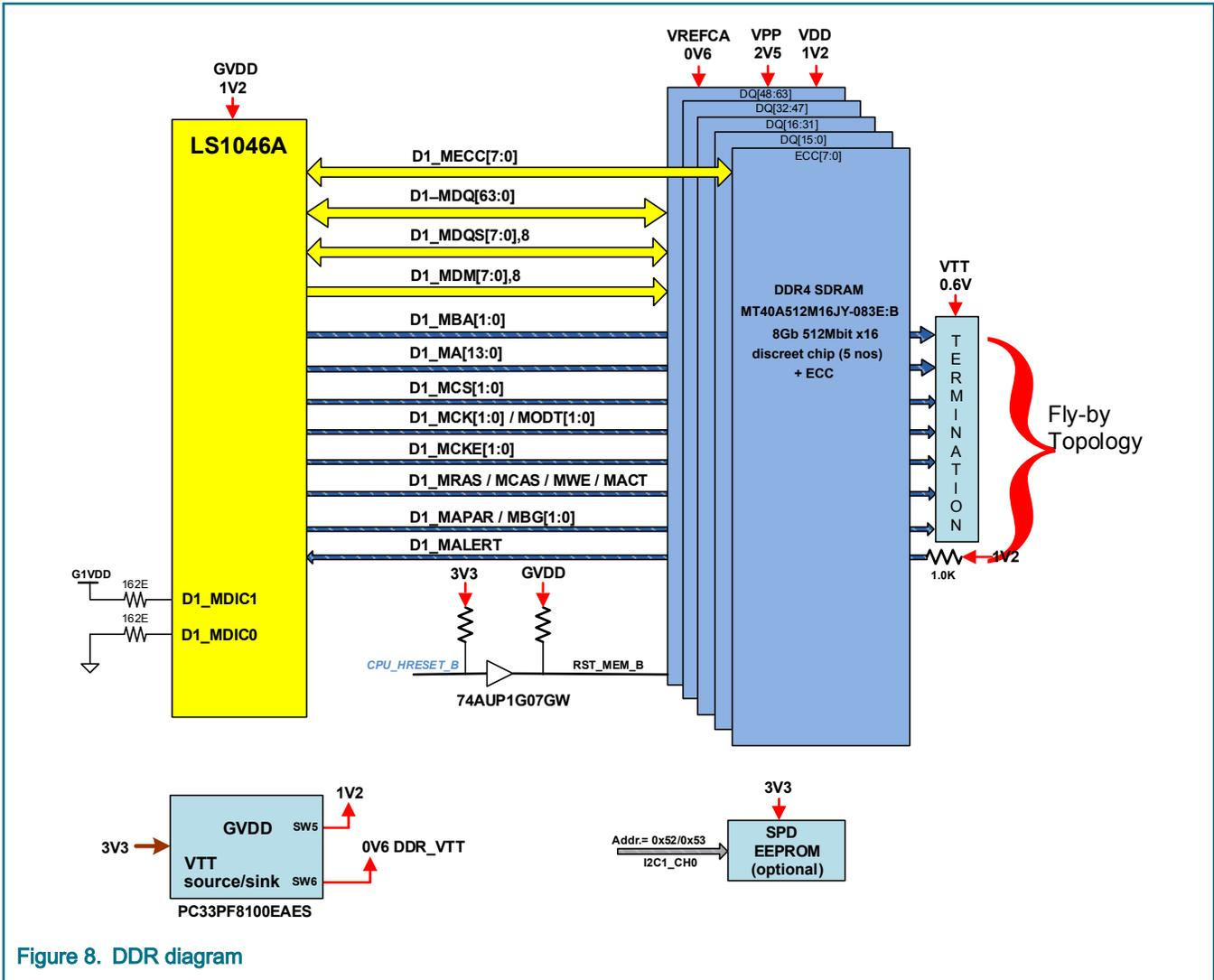
Figure 8. DDR diagram
