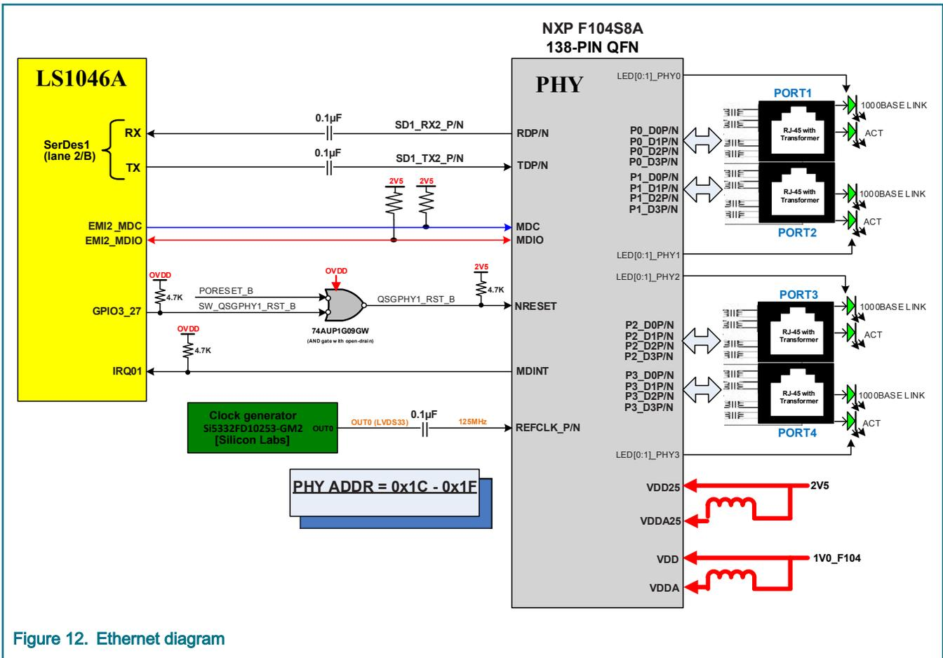
Figure 12. Ethernet diagram
