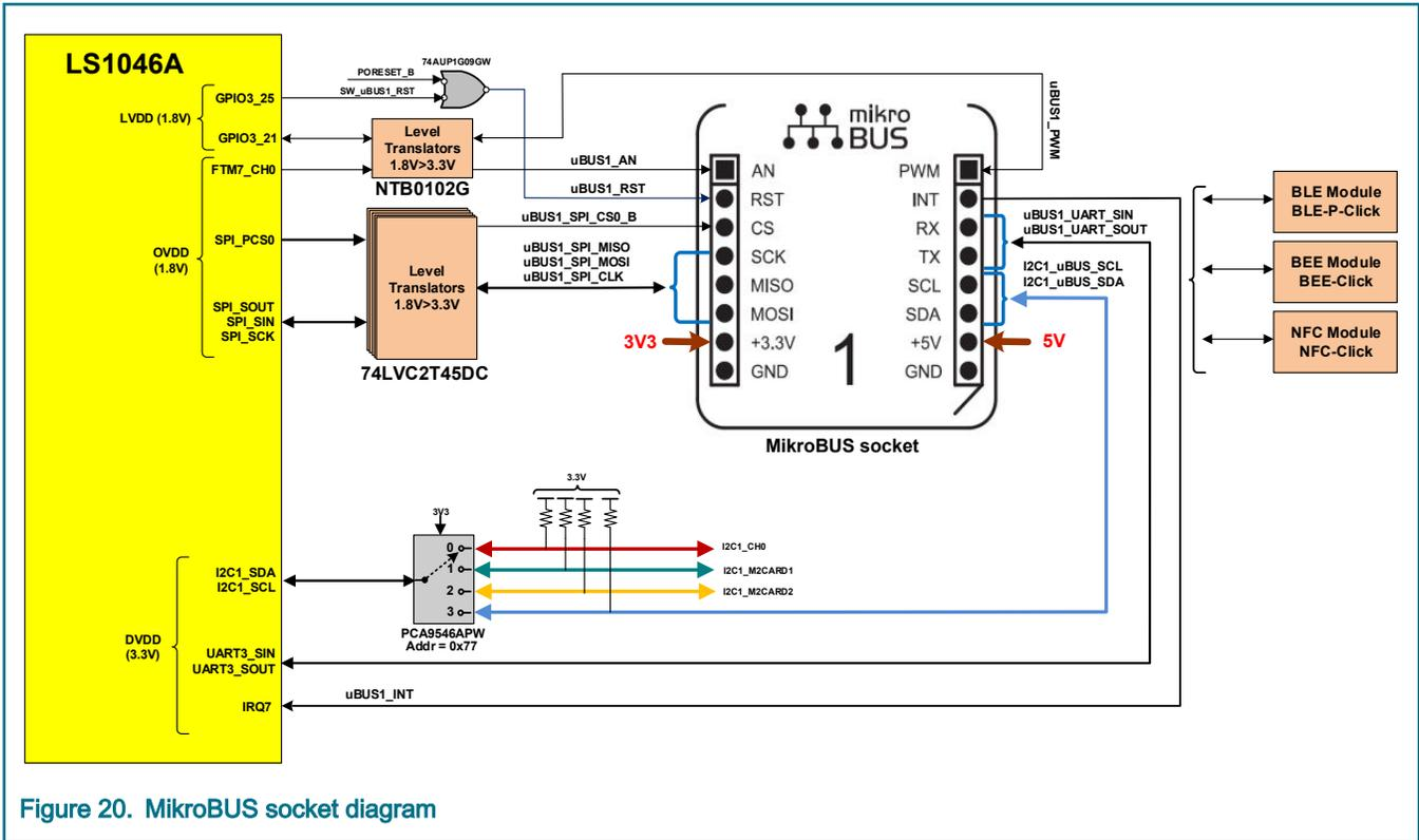
Figure 20. MikroBUS socket diagram
