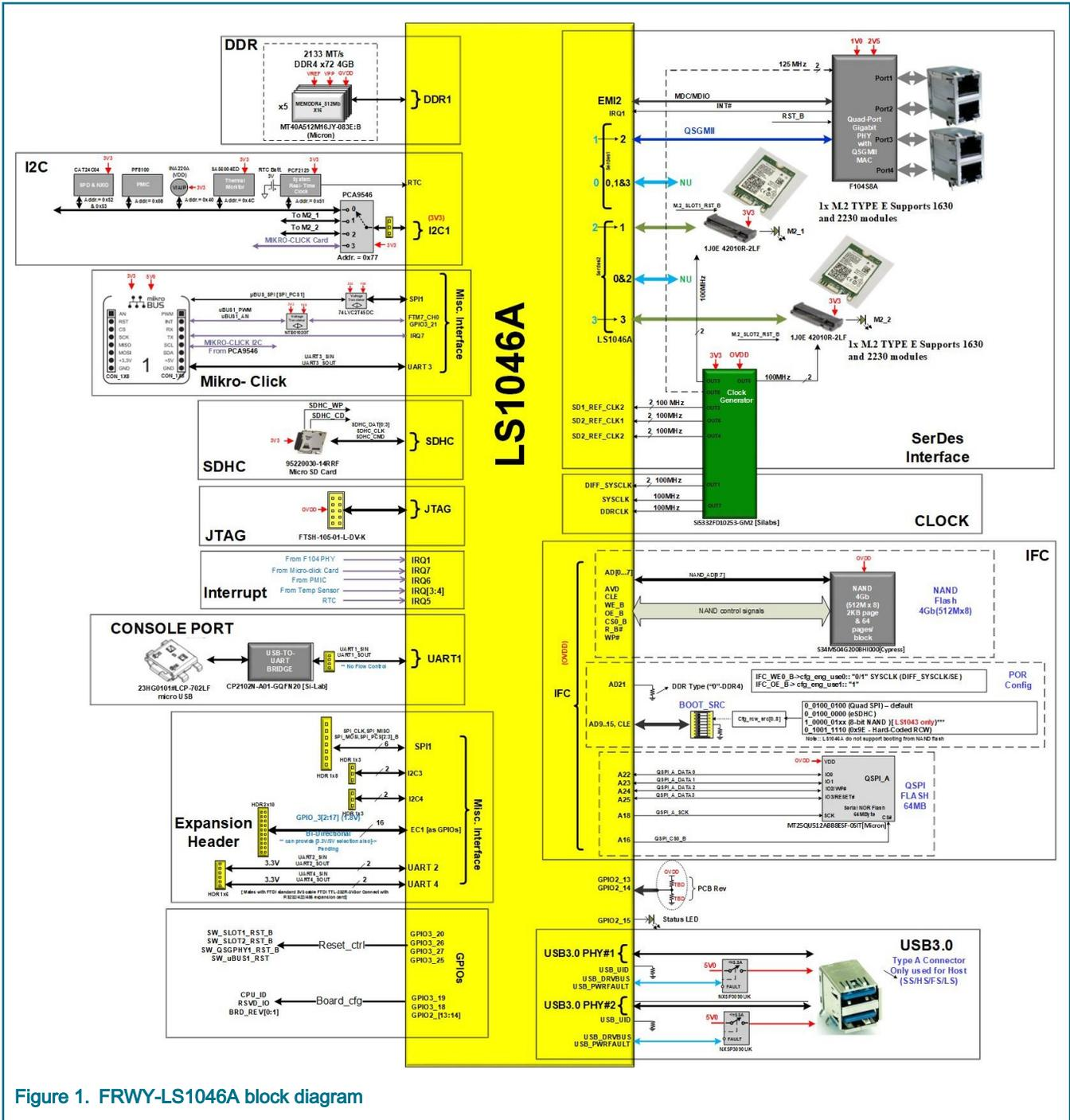
Figure 1. FRWY-LS1046A block diagram
