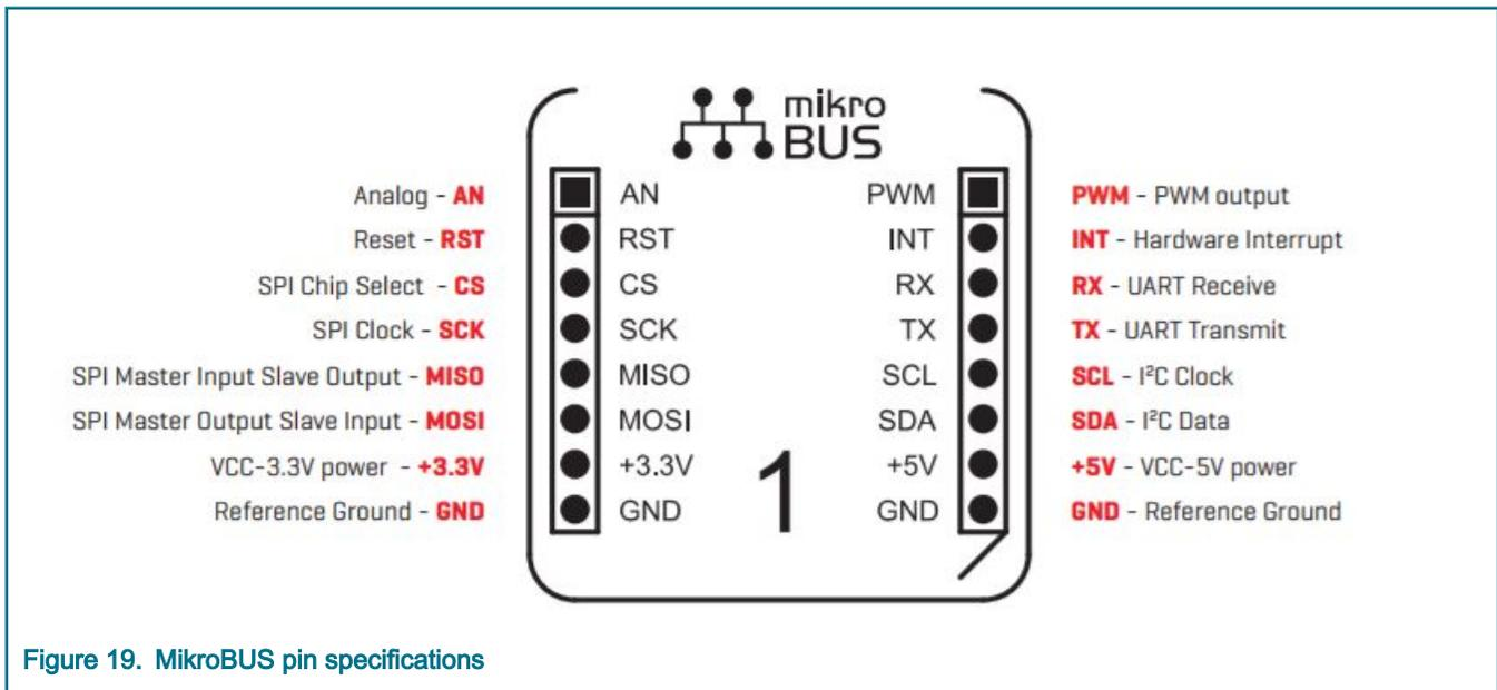
**Figure 19. MikroBUS pin specifications**
