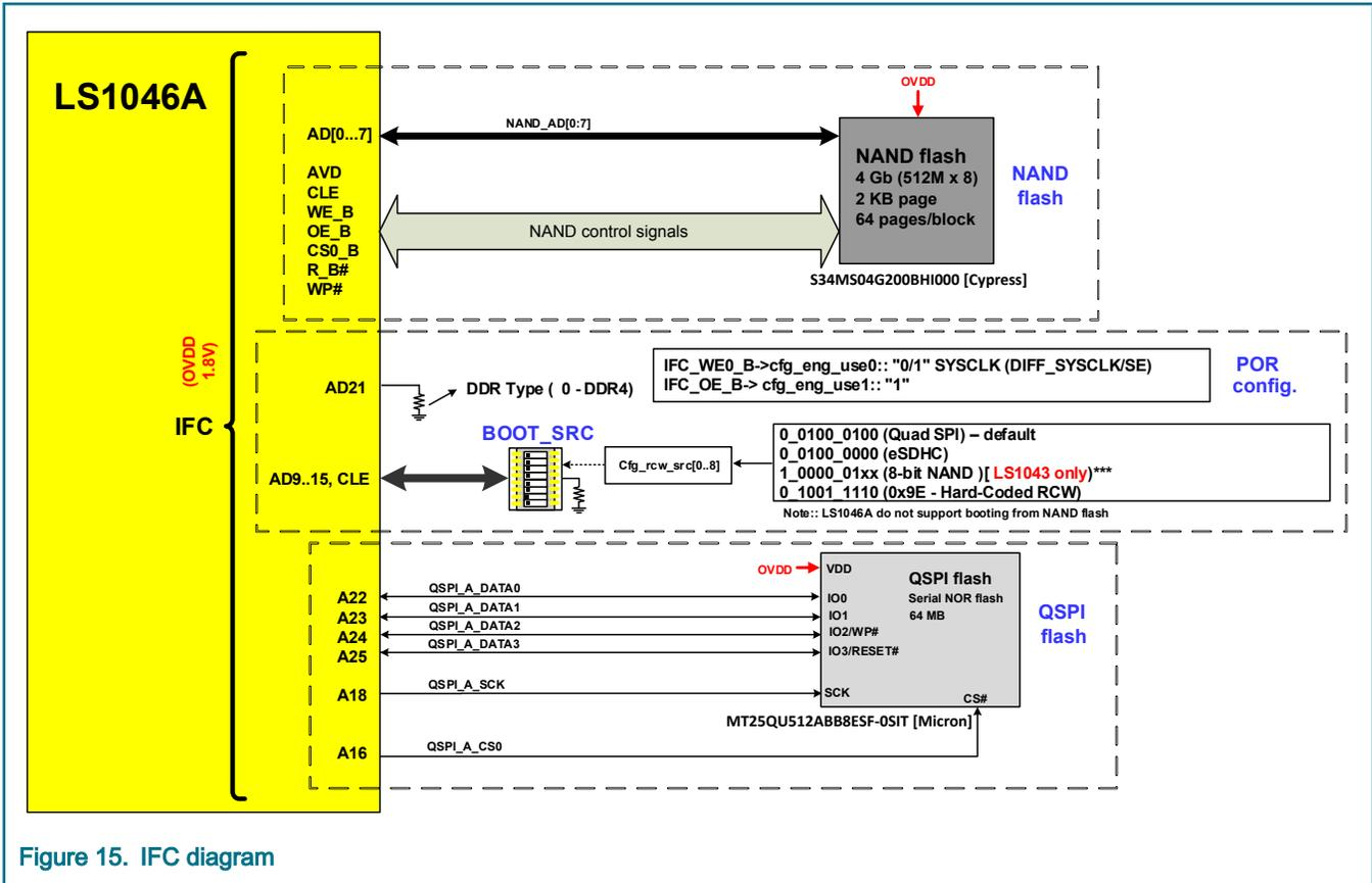
Figure 15. IFC diagram
