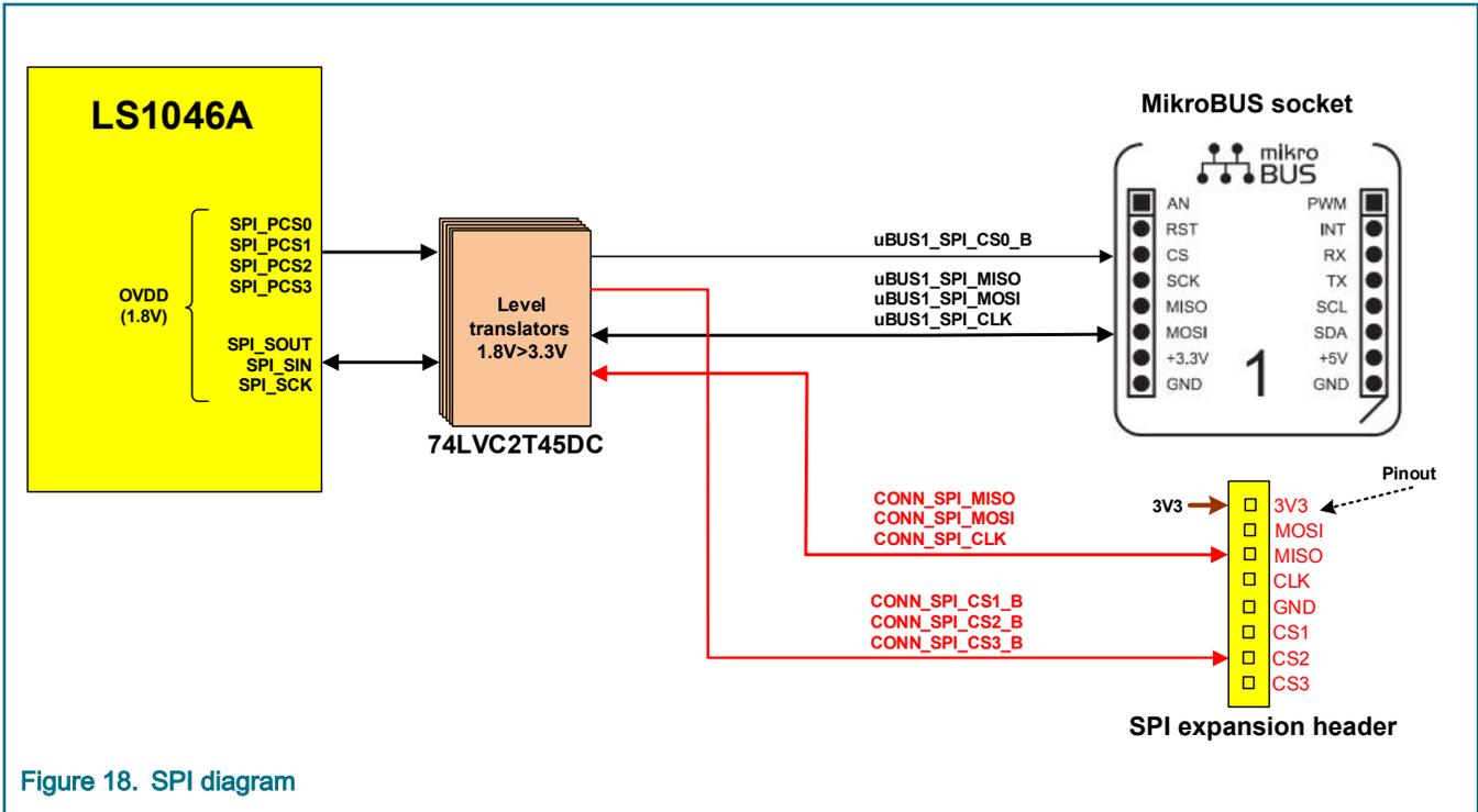
Figure 18. SPI diagram
