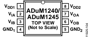
Figure 5. ADuM1240/ADuM1245 8-Lead SOIC (R-8) Pin Configuration
