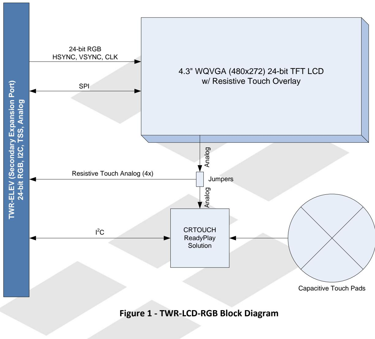
**Figure 1 - TWR-LCD-RGB Block Diagram**
