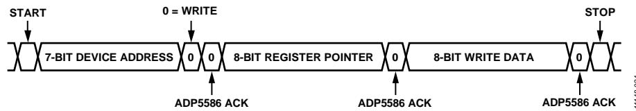
Figure 24. I 2 C Single Byte Write Sequence
