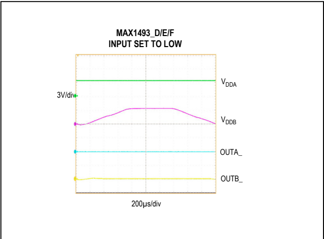
Figure 5. Undervoltage Lockout Behavior (MAX1493_D/E/F Low)
