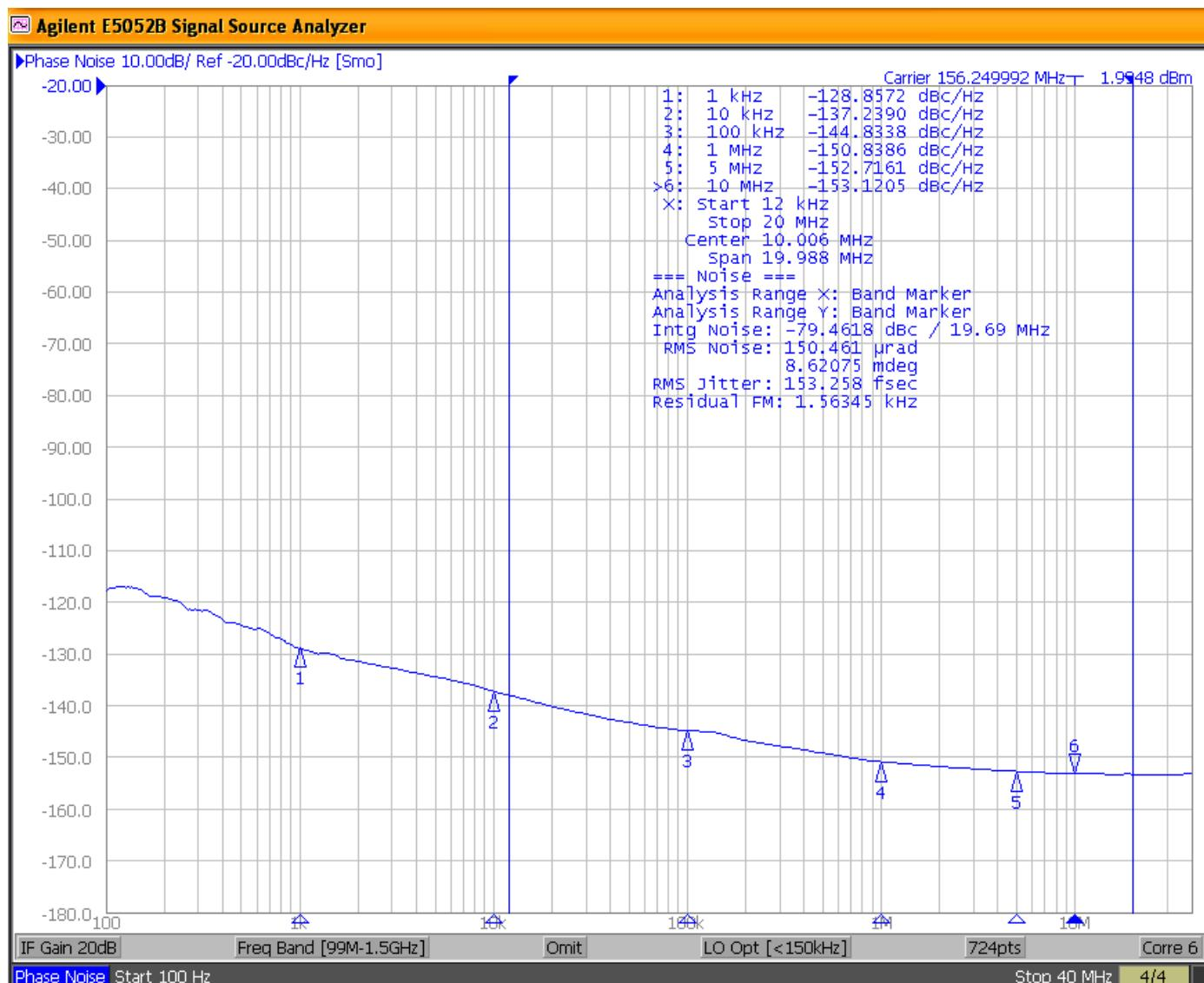
Phase jitter = 153fs<sub>RMS</sub>, 156.25MHz carrier frequency; integration range: 12kHz–20MHz
