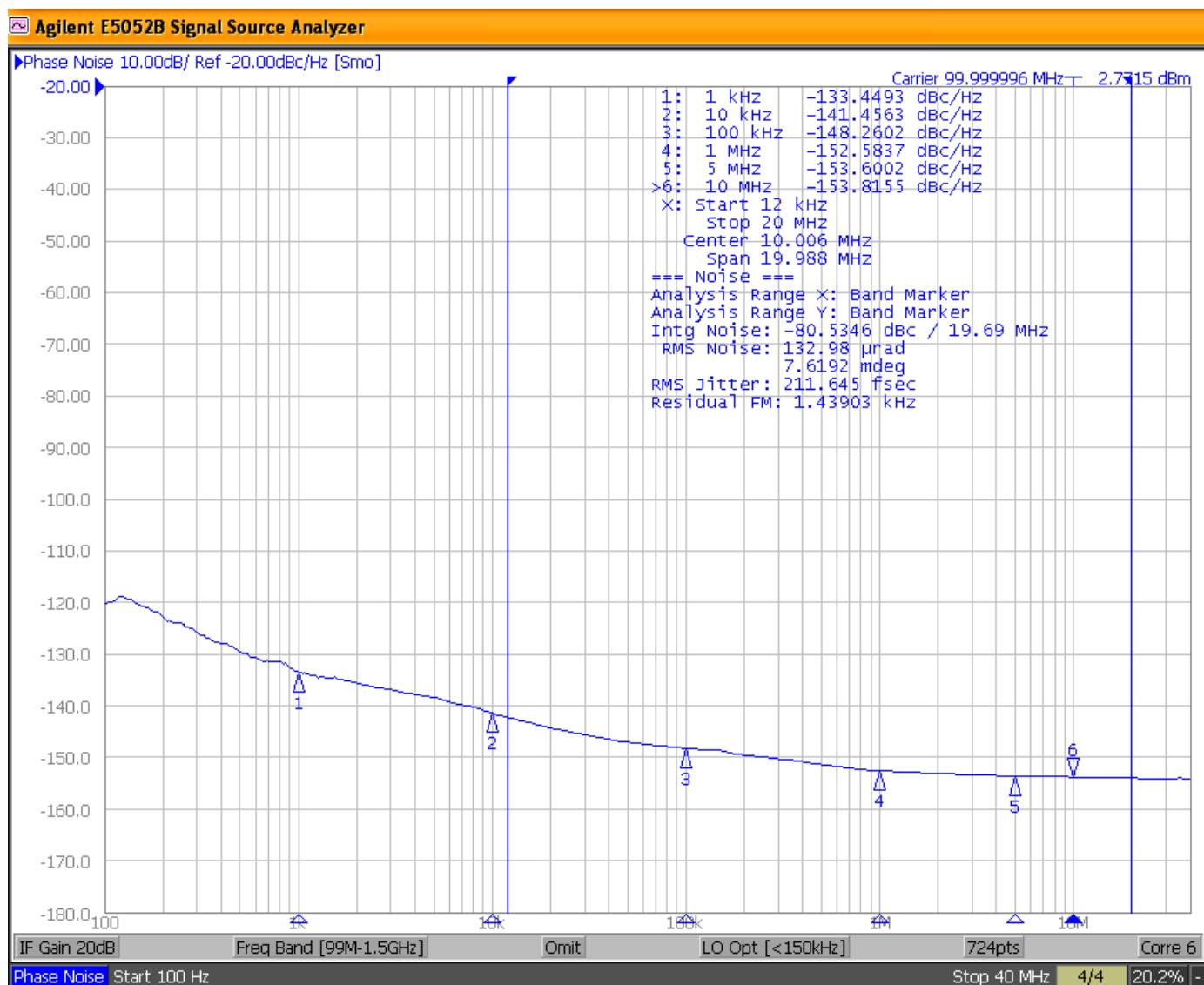
Phase jitter =  $212 \text{ fs}_{\text{RMS}}$ , 100MHz carrier frequency; integration range: 12kHz–20MHz
