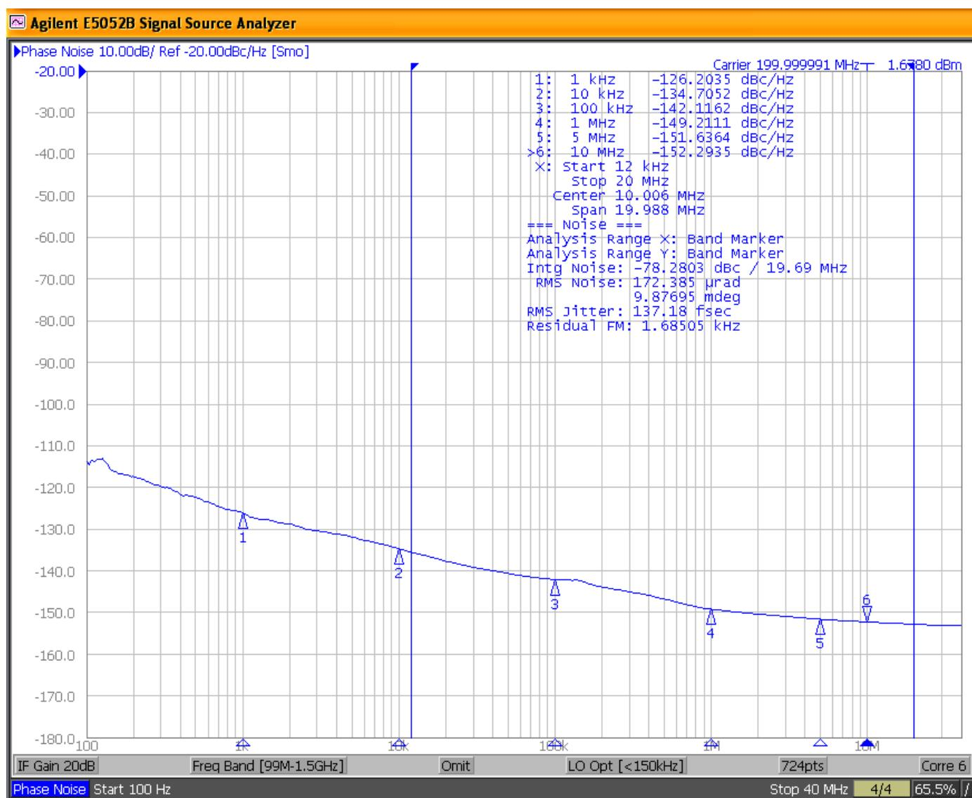
Phase jitter = 137fs<sub>RMS</sub>, 200MHz carrier frequency; integration range: 12kHz–20MHz
