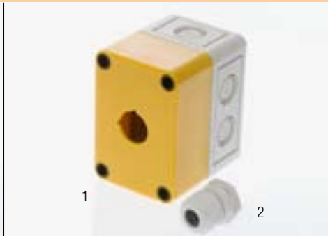
Emergency-stop switch enclosure, with 22.5 mm Ø mounting hole, 94 mm (w) x 65 mm (h) x 81 mm (d), anti twist hole. Cable gland M20, IP66
