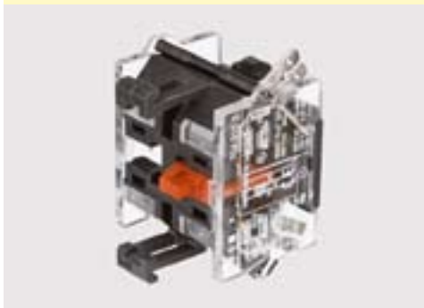
Switching element, plug-in terminal, 6.3 mm, slow-make with forced opening silver contacts
