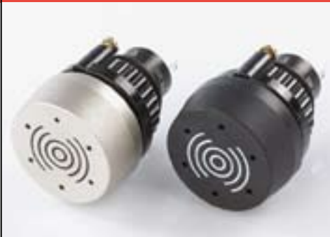
Buzzer, raised, 22.5 mm mounting, IP65, 24VDC, 95dB ±8 at a distance of 0.1m
