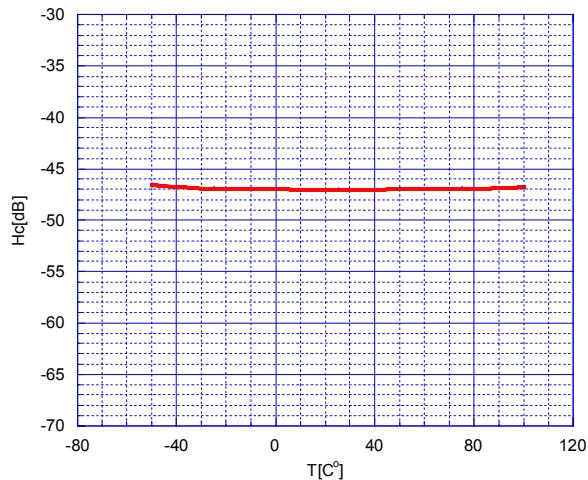
2<sup>nd</sup> Distortion vs. Temperature
