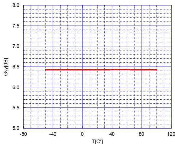
Voltage Gain(C mode) vs. Temperature
