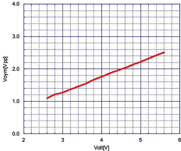
Maximum Output Voltage vs. Operating Voltage
