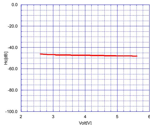
2<sup>nd</sup> Distortion vs. Operating Voltage
