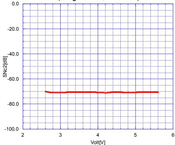
S/N Ratio vs. Operating Voltage
