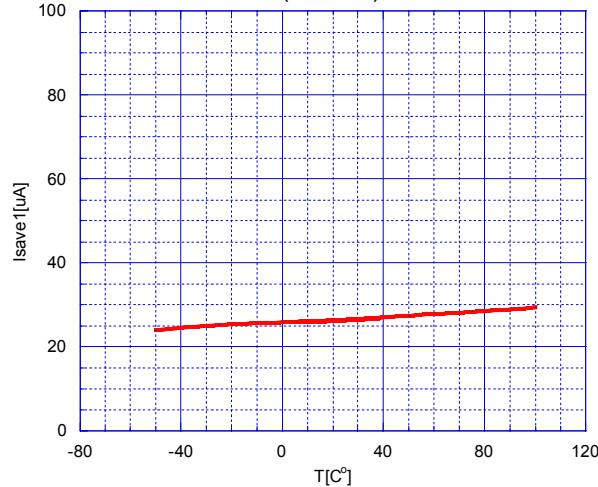
Operating Current2 at Power Save Mode vs. Temperature
