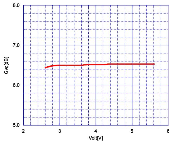
Voltage Gain(V mode) vs. Operating Voltage
