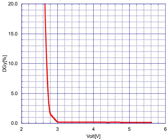
Differential Phase vs. Operating Voltage
