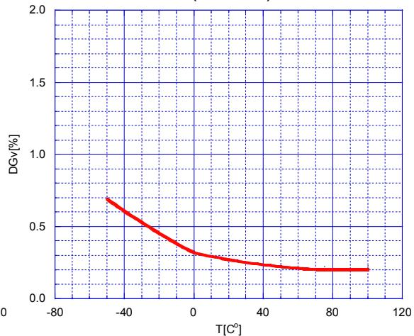
Differential Phase(V mode) vs. Temperature
