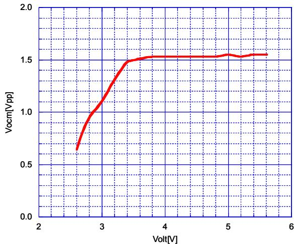
Maximum Output Voltage vs. Operating Voltage
