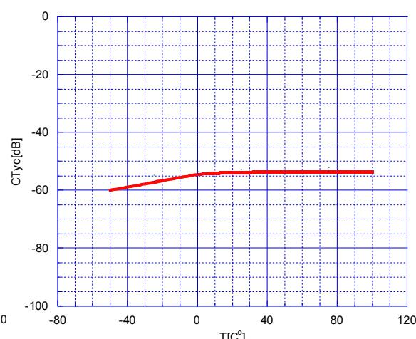
**■TYPICAL CHARACTERISTICS**Closstalk vs. Temperature
