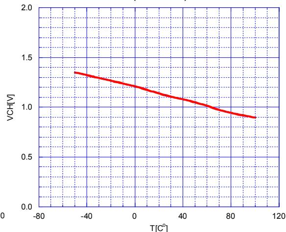
SW Threshold(Low) vs. Temperature
