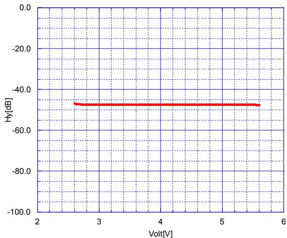
2<sup>nd</sup> Distortion vs. Operating Voltage
