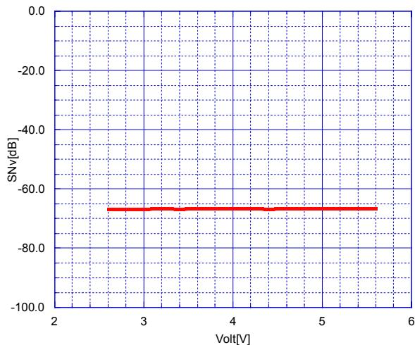
2<sup>nd</sup> Distortion vs. Operating Voltage
