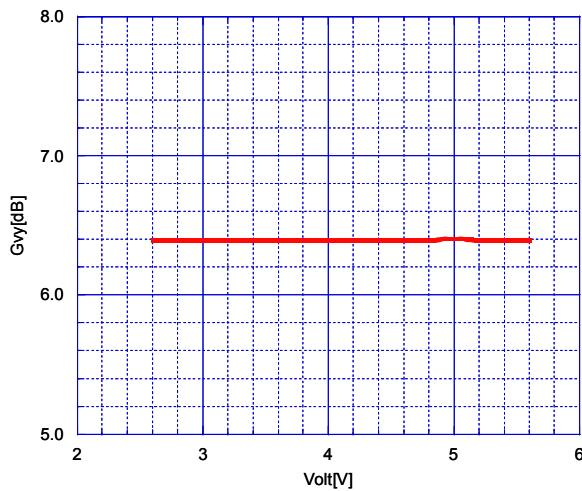
Voltage Gain(C mode) vs. Operating Voltage
