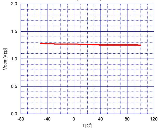
Maximum Output Voltage(V mode) vs. Temperature
