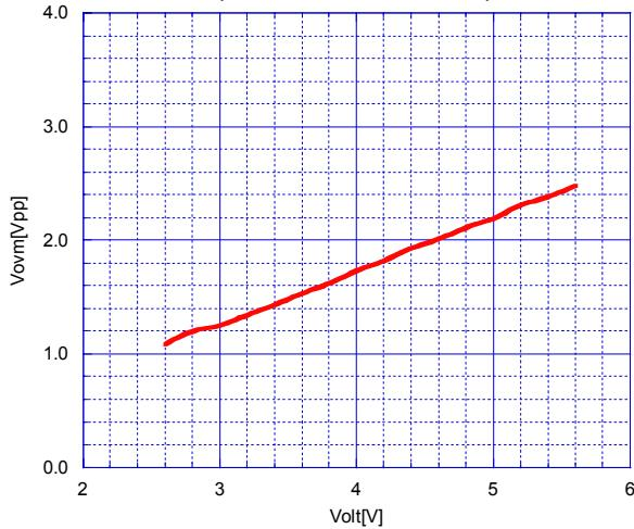
Differential Gain vs. Operating Voltage
