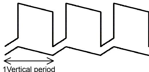
SAG correction circuit generates a low frequency component signal amplified to Vout terminal. Changes of the luminance signal will be low-frequency components, if you want to output a large signal luminance changes. Therefore, generate correction signal of change of a luminance signal to Vout pin. At this time, signal is over the dynamic range of Vout pin. This may cause a lack of sync signal, and waveform distortion.
