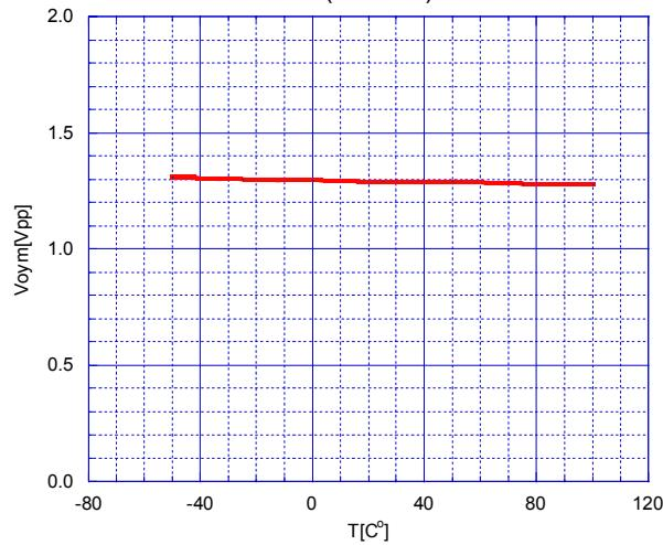
Maximum Output Voltage(Y mode) vs. Temperature
