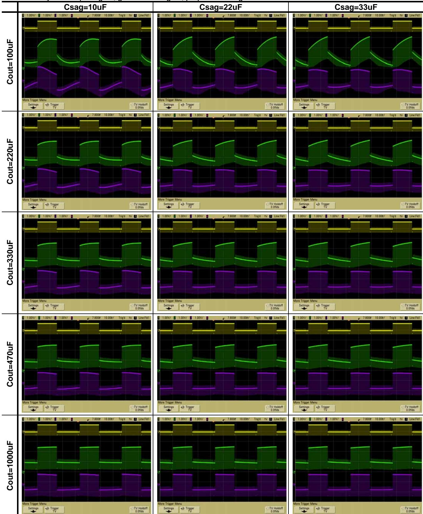
&lt; Not using SAG correction circuit &gt;
