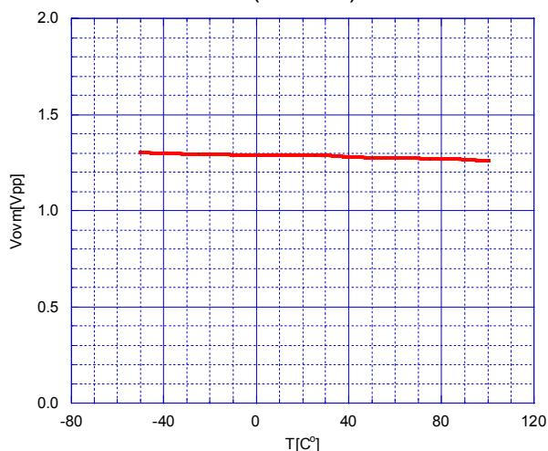
Differential Gain(Y mode)vs. Temperature
