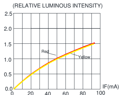
FIG.2 RELATIVE LUMINOUS INTENSITY VS. FORWARD CURRENT
