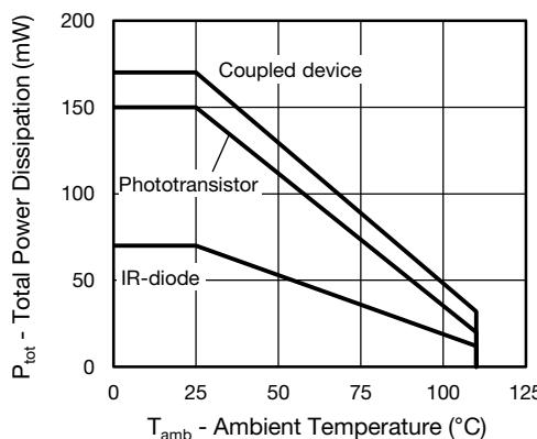
Fig. 1 - Total Power Dissipation vs. Ambient Temperature
