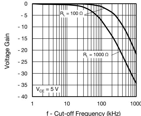
Fig. 16 - Voltage Gain vs. Cut-off Frequency
