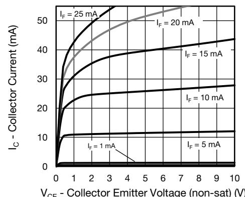
Fig. 5 - Collector Current vs. Collector Emitter Voltage (non-saturated)
