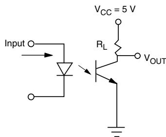
Fig. 2 - Test Circuit
