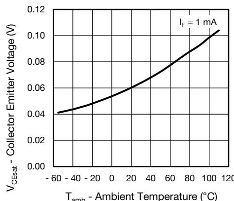
Fig. 8 - Collector Emitter Voltage vs. Ambient Temperature (saturated)
