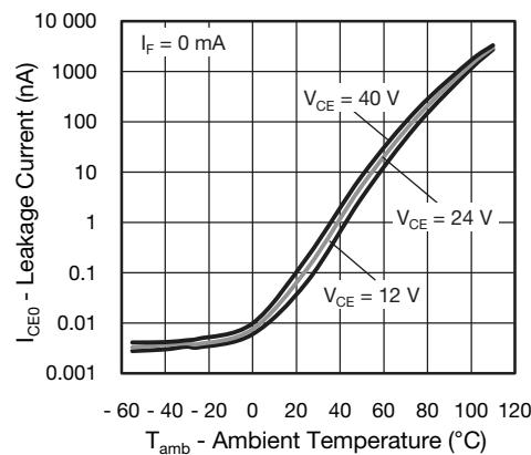
Fig. 6 - Collector Emitter Current vs. Ambient Temperature
