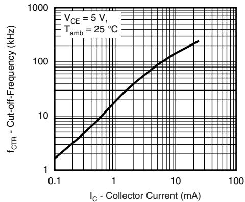
Fig. 13 - Cut-off Frequency (- 3 dB) vs. Collector Current
