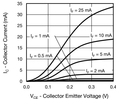
Fig. 7 - Collector Current vs. Collector Emitter Voltage (saturated)
