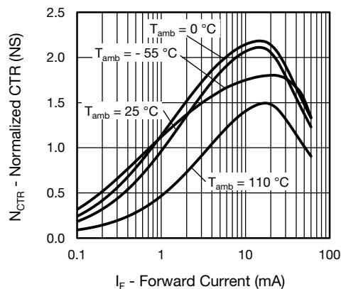
Fig. 12 - Current Transfer Ratio vs. Forward Current (non-saturated)
