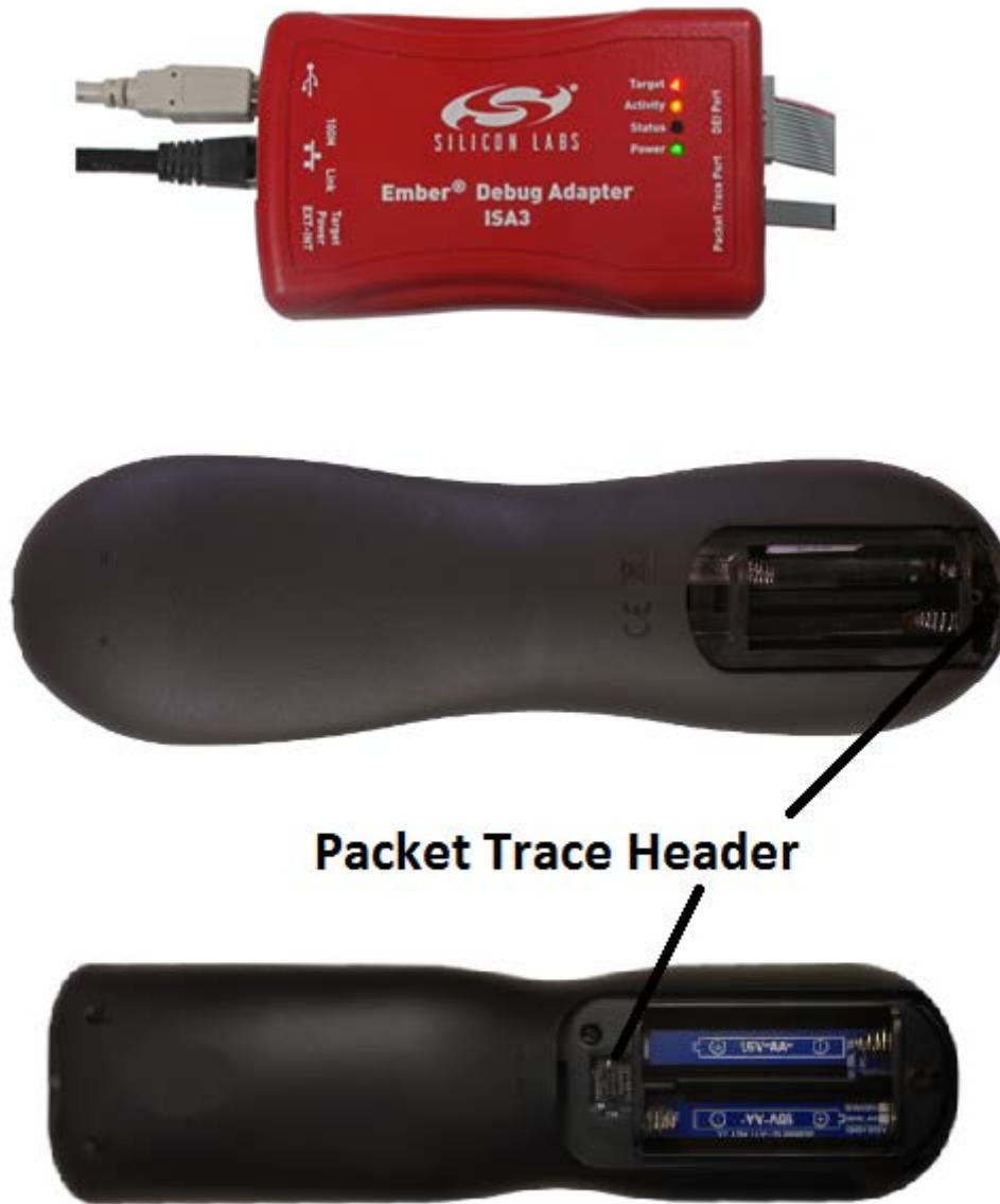
Figure 13. Ember Debug Adapter (ISA3) Connecting Packet Trace to Remote Control for programming
