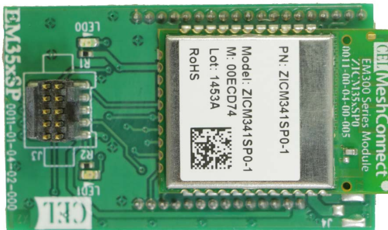
Figure 16. Module with PCB Antenna
