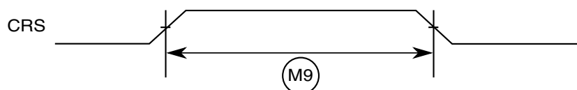
Figure 43. MII async inputs timing diagram
