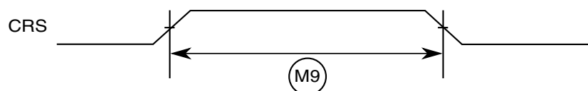
Figure 43. MII async inputs timing diagram
