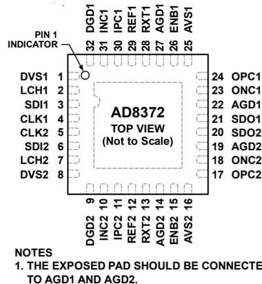
Figure 4. Pin Configuration
