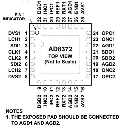
Figure 4. Pin Configuration
