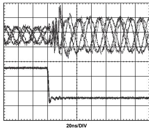
Figure 13. AD8372 Response to 6 dB Step Change in Gain (Gain Register Setting 36 to Setting 42); Falling Edge Shown is Serial Clock Input Edge
