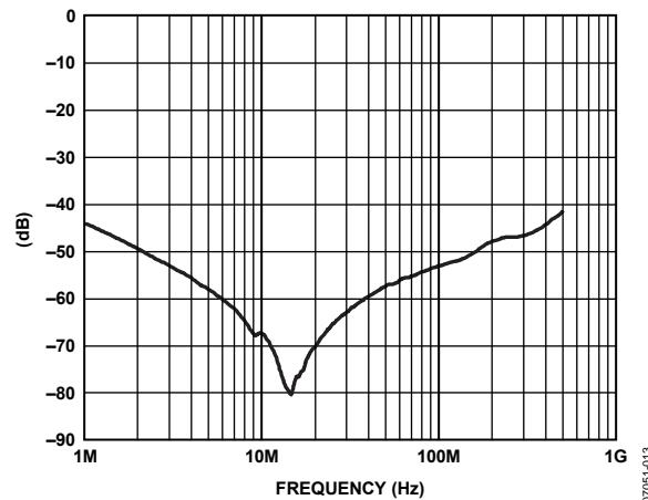
Figure 12. Isolation, Input to Opposite Output at Maximum Gain
