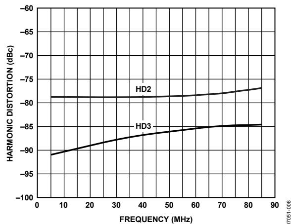
Figure 6. 2<sup>nd</sup> and 3<sup>rd</sup> Harmonic Distortion
