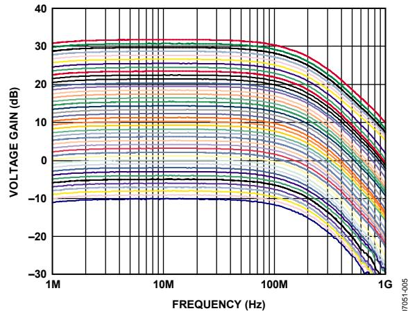
Figure 5. Gain vs. Frequency by Gain Code (All Codes),
