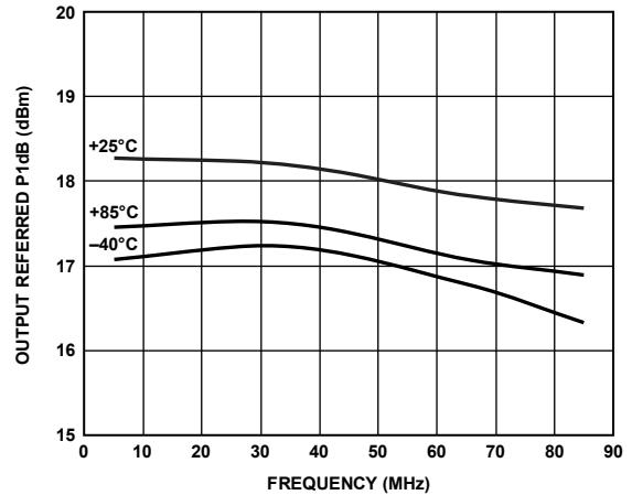
Figure 8. P1dB, Maximum Gain
