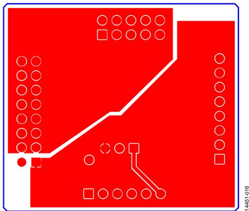
Figure 16. EVAL-AD5321DBZ Daughter Board Bottom Side Routing
