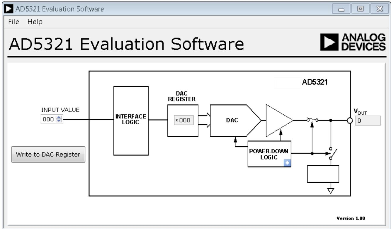
Figure 4. AD5321 Evaluation Board Software Main Window
