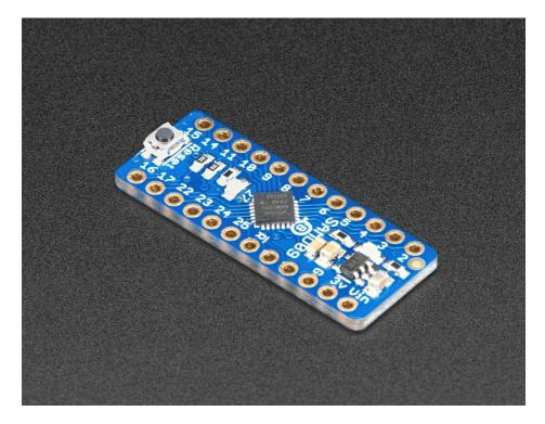
The ATSAMD09 breakout is great for development of seesaw capabilities (we use it in-house for our design work) or you can use it as-is to give your Raspberry Pi or ESP8266 more hardware support! Each breakout comes with the assembled and tested board, as well as some header strips.
