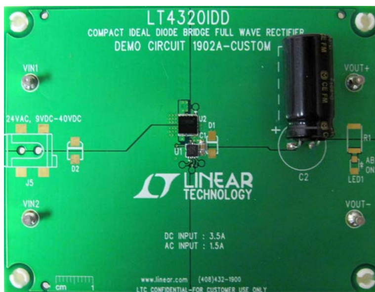
Figure 4. Demonstration Circuit 1902A Used in Figure 3 Thermograph
