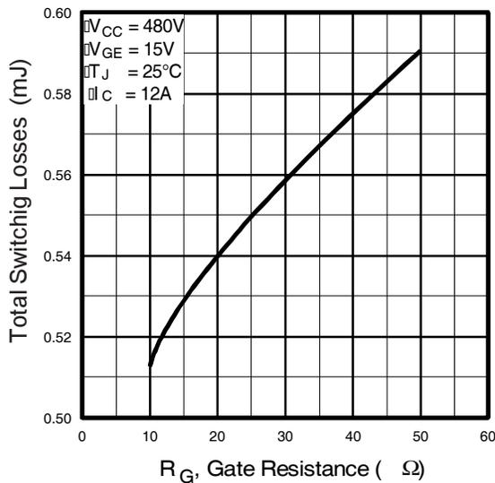
**Fig. 9** - Typical Switching Losses vs. Gate Resistance
